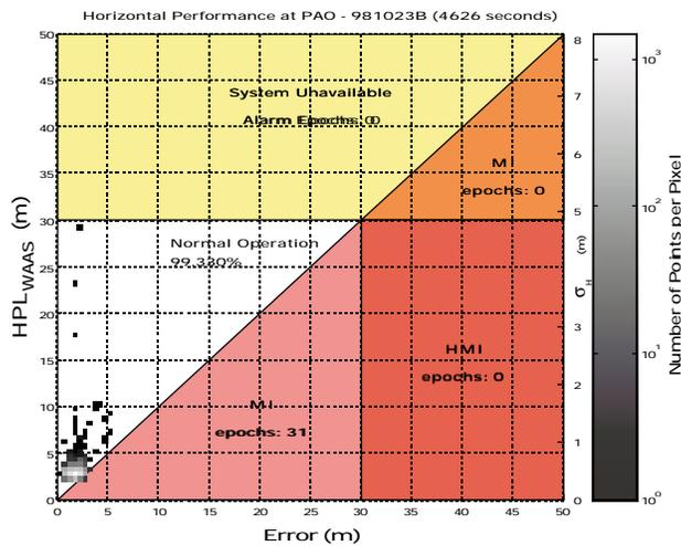
Figure 12. Horizontal Results when GEO Satellite with Highest Power (SNR) Selected as Primary Signal.
