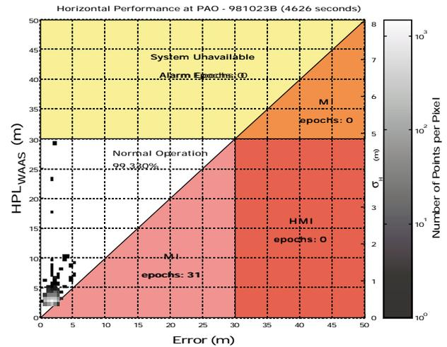
**Figure 8. Flight Test Results Using the Stanford SNR-Based Receiver Noise Model.**
