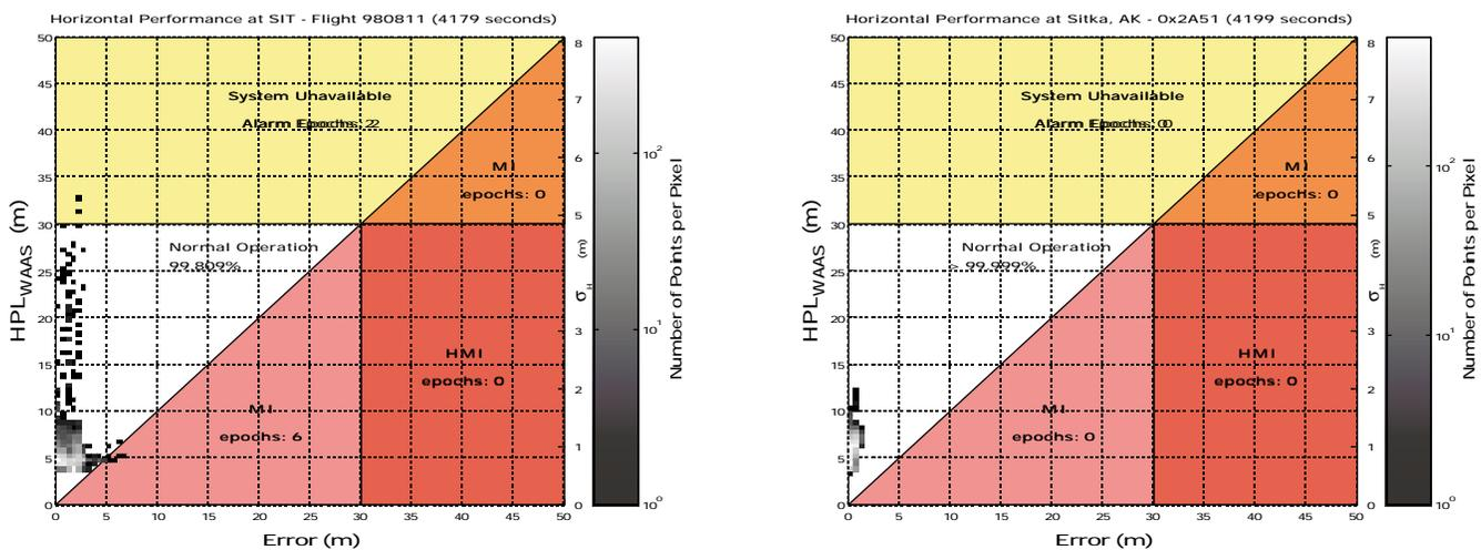
Figure 9. Comparison of Flight (Left) and Static (Right) Horizontal Results at Sitka. Note the effect in flight of message loss on the HPL and the modeling errors in horizontal error.
