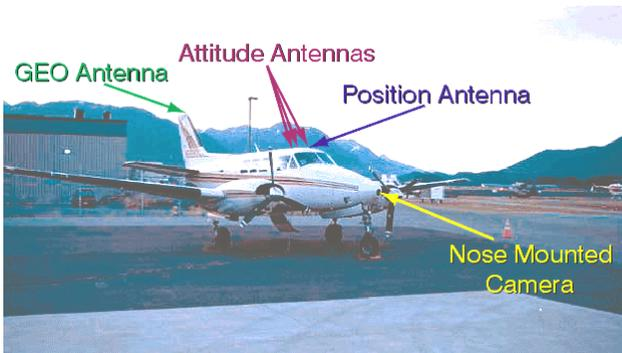
**Figure 4. Aircraft Used in Flight Tests.**
