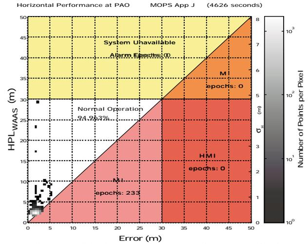
**Figure 7. Flight Test Results Using the MOPS Appendix J Model for Receiver Noise.**
