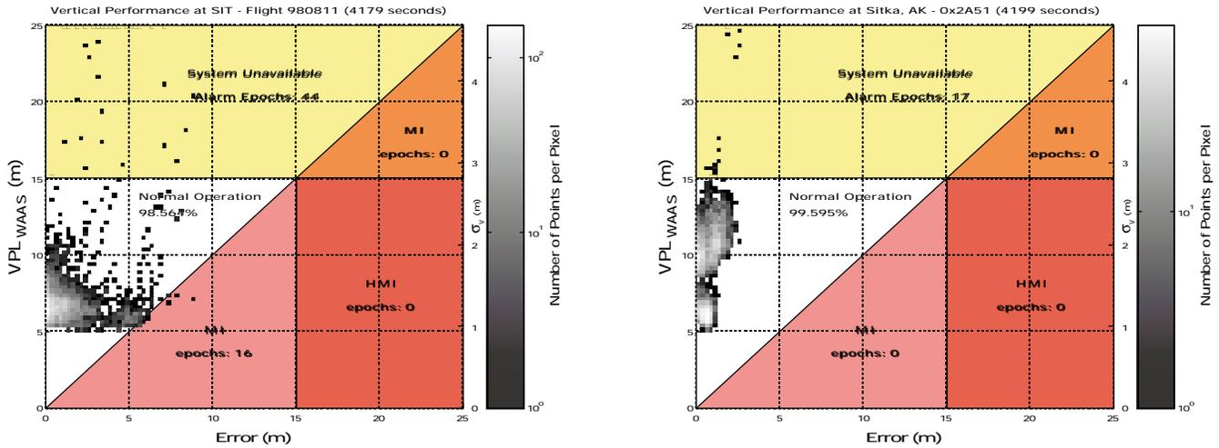
**Figure 10. Comparison of Flight (Left) and Static (Right) Vertical Results at Sitka. Note the effect in flight of message loss on the HPL and the modeling errors in horizontal error**
