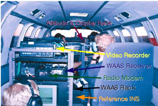
**Figure 3. Equipment Setup Inside Cabin.**
