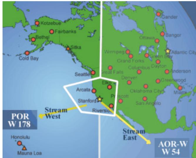
**Figure 13. Diagram of Stations Used for Interoperability Flight.** Stations to the left were used to drive POR and stations to the right were used to drive AOR-W. The stations indicated in the middle were common to both to ensure ionospheric corrections (Stanford passive).
