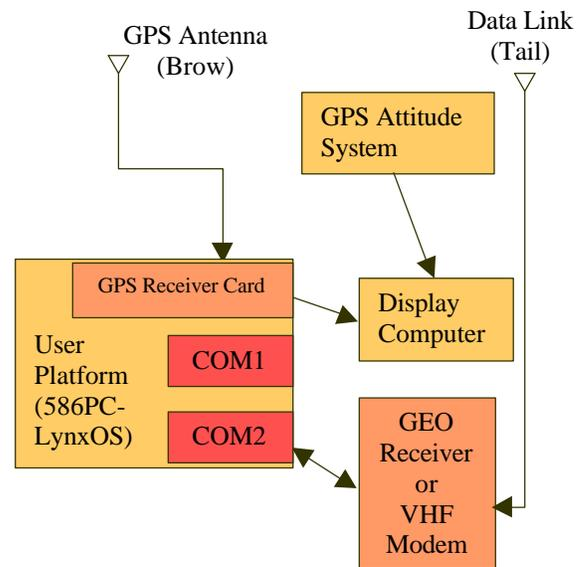
**Figure 2. User Platform Setup During Flight Tests in Sitka, Alaska and Palo Alto, California**
