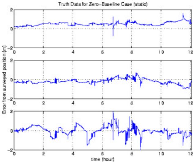
**Figure 6. DDSCMC Minus Surveyed Position for Twelve Hours. Errors are in East, North and Up components.**
