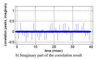
Figure 7. Correlation of the Compass E2 signal with a slice of itself
