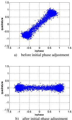
Figure 9. Compass E2 signal I-channel time-domain scatter plot
