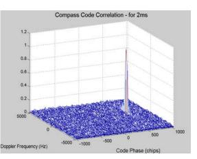
Figure 12. Acquisition plot of Compass-M1 E2 I-channel
