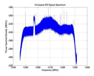
Figure 6. Unaveraged Spectrum of Compass-M1 E6
