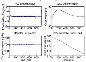
Figure 13. Tracking results of Compass-M1 E2 I-channel
