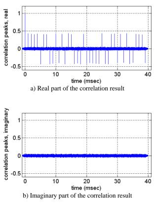
Figure 8. Correlation of the Compass E2 signal with a slice of itself, after Doppler wipeoff
