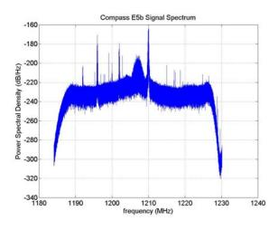
Figure 5. Unaveraged spectrum of Compass-M1 E5b
