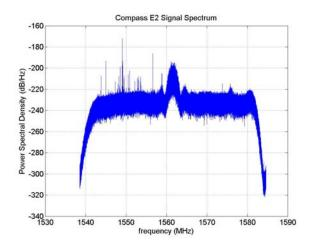
Figure 4. Unaveraged spectrum of Compass-M1 E2
