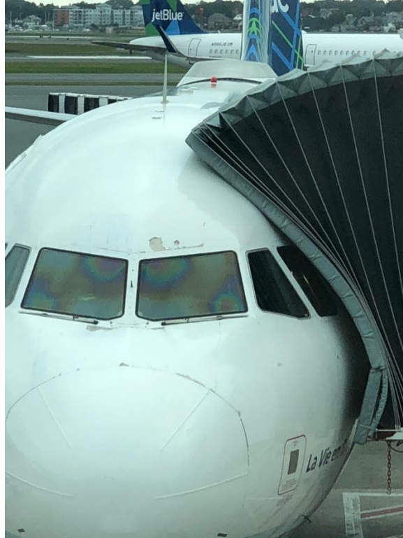
Figure 10. Airbus A320 with Two GPS Antennas Visible atop Fuselage
