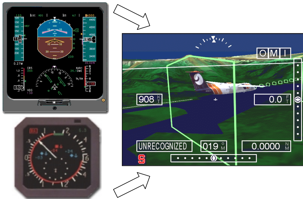
Figure 1. A Honeywell Primary Flight Display and a TCAS 2000 display can be integrated into an intuitive graphical image.
