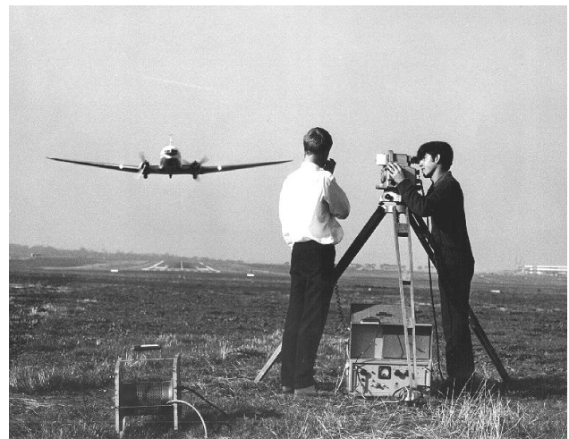
Figure 1: The two surveyors on the ground measure the aircraft's deviation from the desired flight path using a theodolite (courtesy of CAHS collection) [5]
