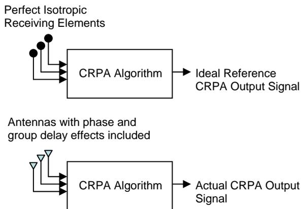
**Figure 12. Flowchart for CRPA signal simulation**
