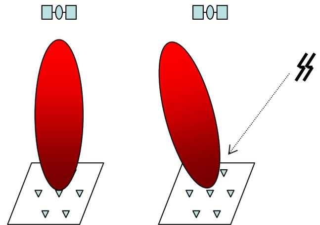
Figure 11. Deterministic beam forming vs. adaptive processing
