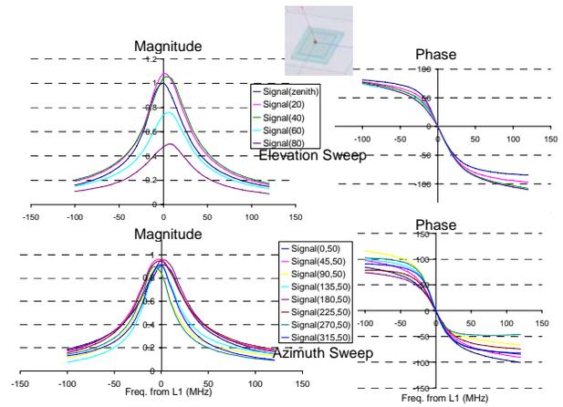
Figure 5. Frequency response of single antenna with sweep in incident signal direction: magnitude and phase responses
