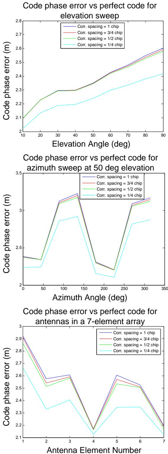
**Figure 9. Code phase errors for different correlator tracking pair spacings**
