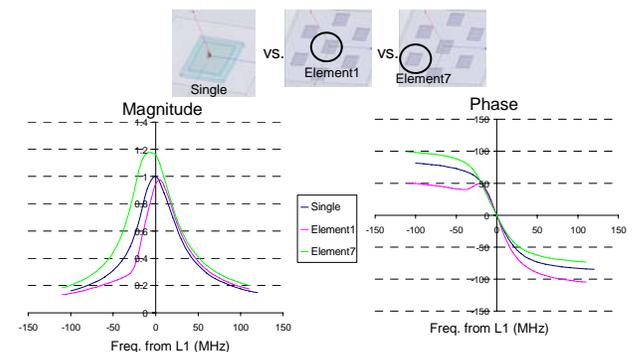
Figure 6. Frequency response comparison of single antenna vs. different antenna elements in a 7 element CRPA: magnitude and phase responses
