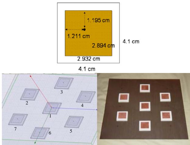
**Figure 2. Single probe fed rectangular patch antenna and 7 element array**
