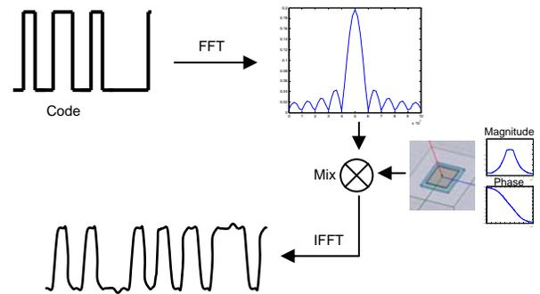
**Figure 3. Antenna group delay effect on code**
