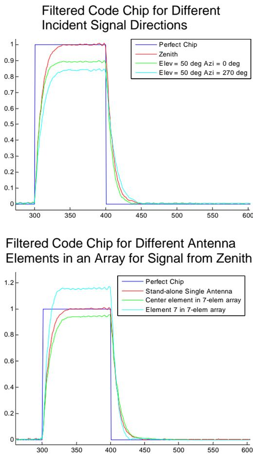
**Figure 7. Antenna frequency response effect on code chip**
