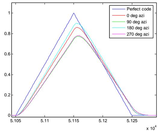
**Correlation Peak Distortion for Antenna Elements in an array (Signal from Zenith)**
