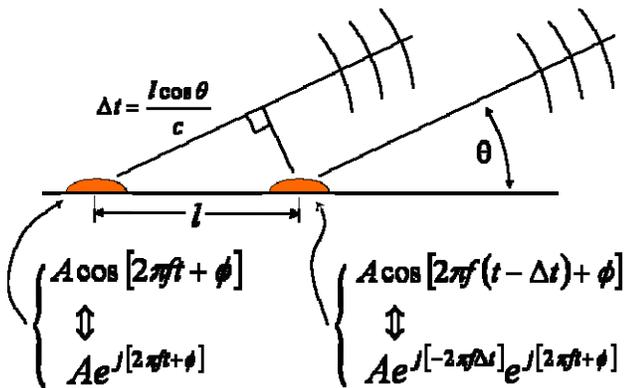
Figure 10. Phased array beam forming
