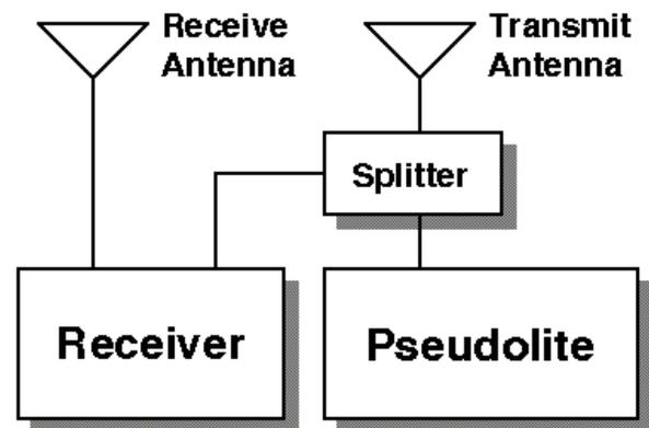
Figure 2: Transceiver Architecture
