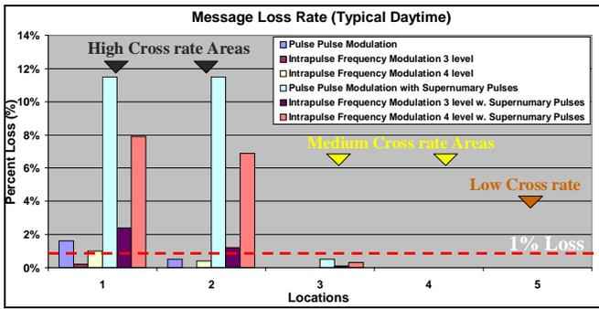
Figure 12. Message Loss Rates with Cross Rate Interference Only (No Sky wave Interference)
