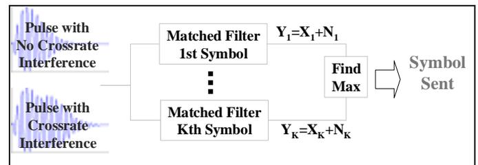
Figure 4. General Match Filter for Interference and Noise on LORAN
