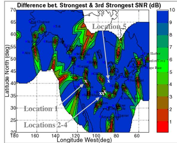
Figure 10. Relative Strength of LORAN interference signals (vs. strongest signal)
