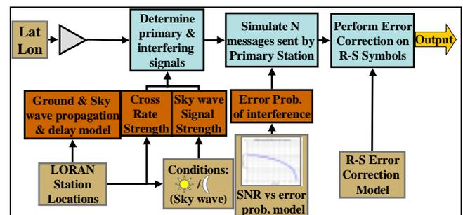
Figure 11. Data Channel Model Flowchart
