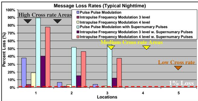
Figure 13. Message Loss Rates with Sky wave Interference
