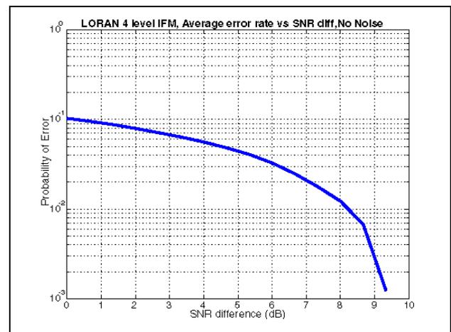
Figure 5. Average Error Rate for Interference from another LORAN signal
