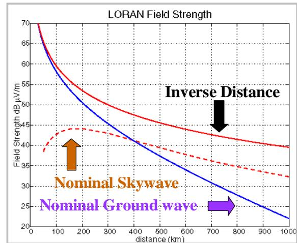
Figure 8. Average Ground wave and Single hop sky wave signal strength
