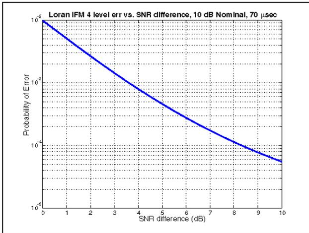
**Figure 6. Error Rate vs. Relative SNR difference for a 10 dB LORAN signal and an interfering signal that is delayed 70 microseconds**
