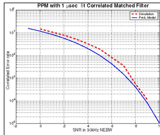
Figure 2. PPM Probability of Symbol Error vs. SNR
