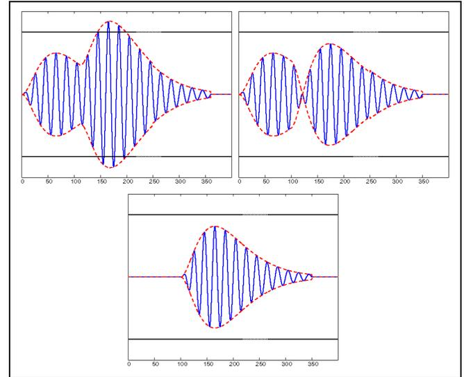
**Figure 7. Modifying the Received Signal. From top left clockwise - 1) Strongest Combined Signal 2) Weakest Combined Signal 3) Modified Signal based on Weakest Combined Signal. Lines represent Nominal value of Sky wave**
