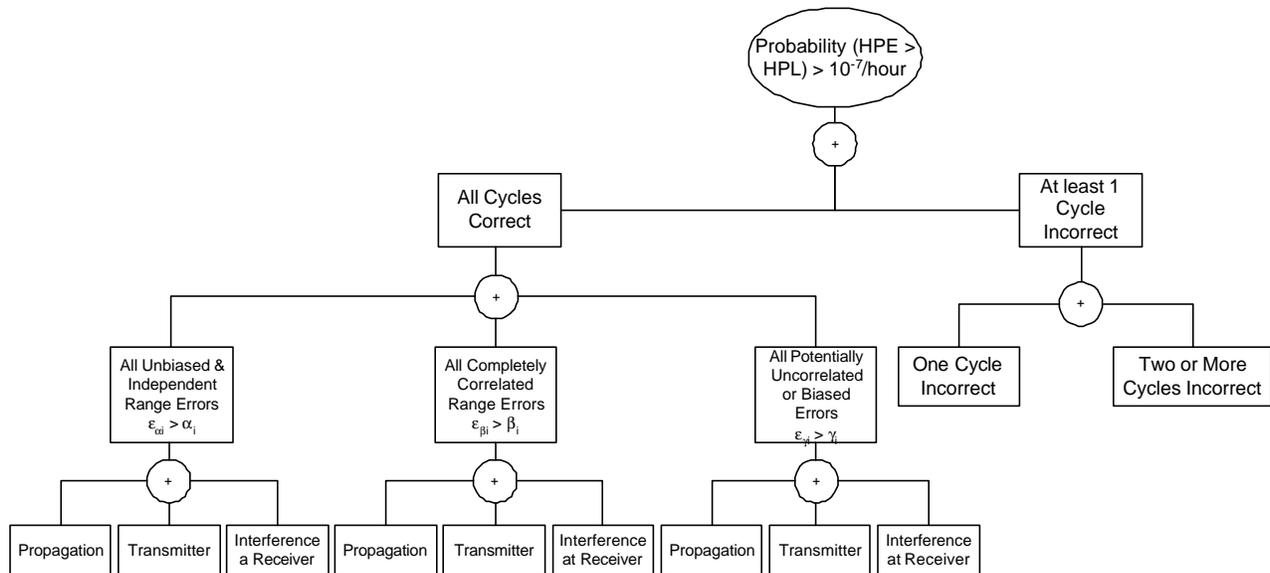
Figure 2. Preliminary High Level Integrity Fault Tree
