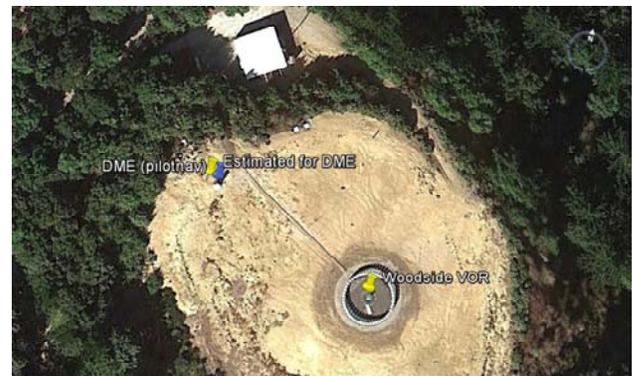
Figure 15. Woodside VORTAC (DME/TACAN Antenna & VOR Antenna)
