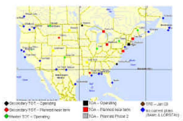
Figure 8. Time of Transmission (TOT)/Time of Arrival (TOA) Monitor Network
