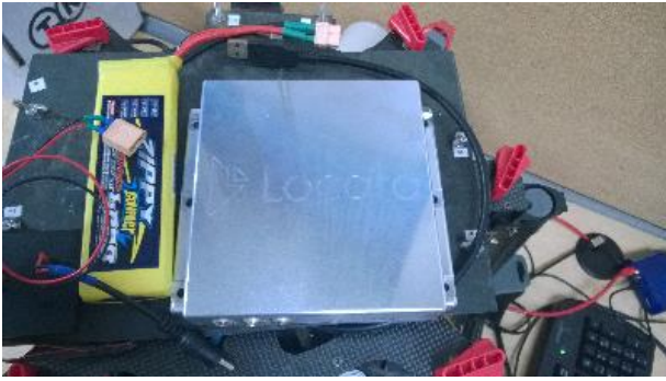
Figure 5: Locata receiver mounted to underside of JAGER
