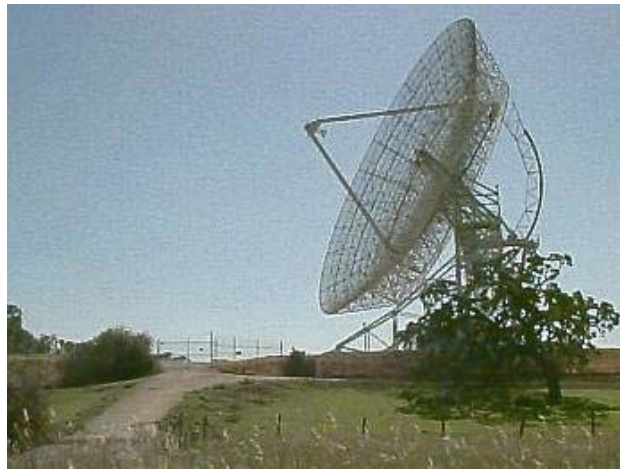
Figure 4. High-gain parabolic radio telescope antenna used to acquire low-noise, wide bandwidth samples of the GPS signals.
