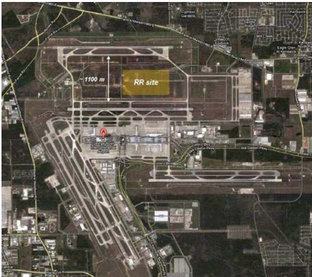
Figure 18: Reference Receiver Siting at Houston/George Bush Airport
