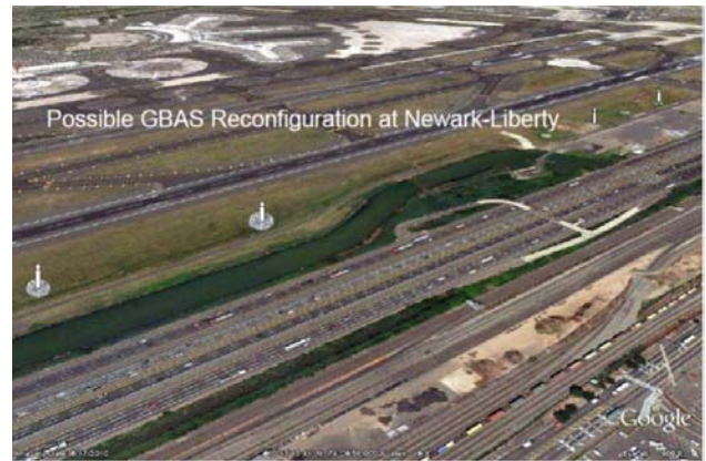
Figure 17: Example Newark Antenna Reconfiguration with Greater Separations
