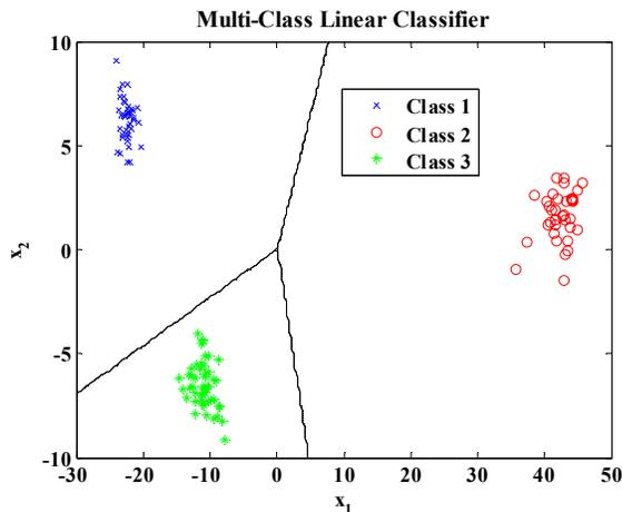
Figure 7. Multi-class linear classifier trained by the Perceptron algorithm
