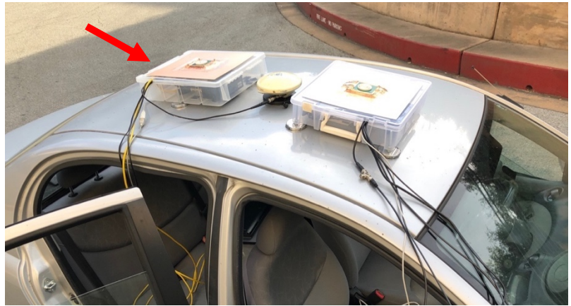
Figure 11: Driving test setup. The DPA is the aft antenna (red arrow), placed on an aluminum ground plane for better reception. The IMU is in the box underneath.
