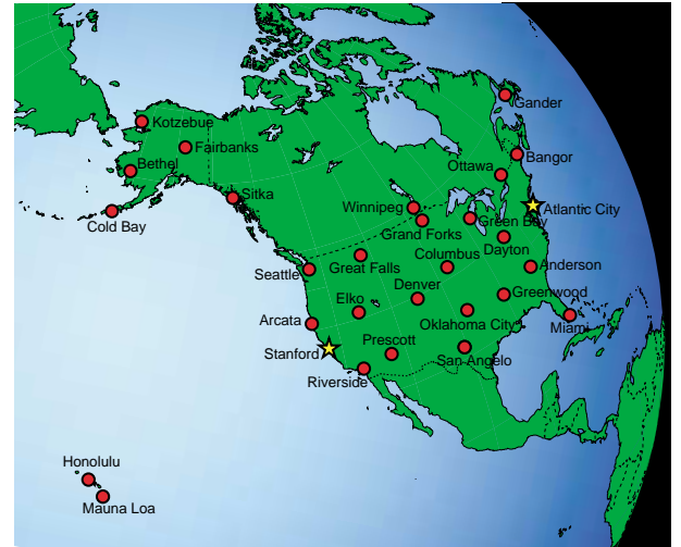
Figure 1. The NSTB network. Each circle represents the location of a reference station. The master stations at the FAA Technical Center and Stanford University are shown as stars. [11]
