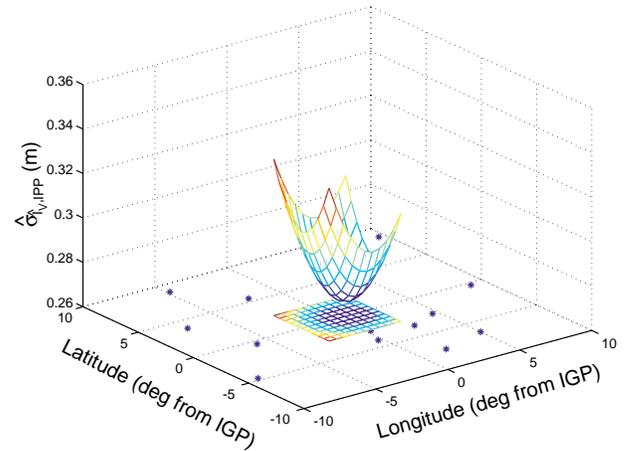
**Figure 8** The location of all IPPs within  $10^\circ$  of the IGP are shown by the blue asterisks. The mesh is the evaluation of (16) for locations within the  $5^\circ$  square surrounding the IGP. Also shown is a projection of this mesh at the bottom. The maximum uncertainty of  $0.35$  m within this square occurs at the Southwest corner. The  $\sigma_{GIVE}$  would need to be at least this large.
