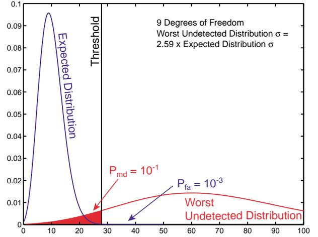
**Figure 3.** The blue trace shows the expected distribution for the chi-square variable. The black line represents the threshold listed in Table 1. The red trace corresponds to the worst case undetectable distribution when all the variances are multiplied by 6.69 with a corresponding  $P_{md} = 10^{-1}$ .
