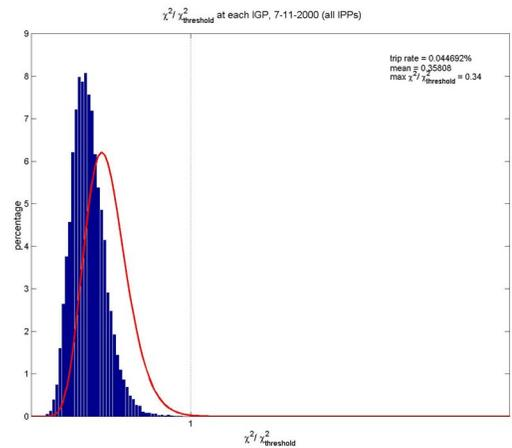
**Figure 10.** Histogram of the chi-square statistic for a quiet day on the prototype system. The red line indicates the theoretical result. Since the noise estimates tend to be conservative, the observed distribution is shifted to the left of the theory.
