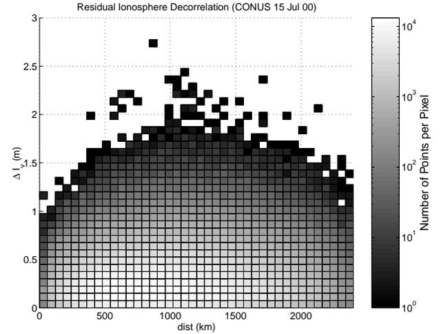
**Figure 9.** A two dimensional histogram representing the distribution of differential vertical delays, after a planar fit has been removed, versus IPP separation. This data is for a severe storm day where the chi-square detector has been used to remove locally disturbed ionosphere. Compare to Figures 1 and 2.
