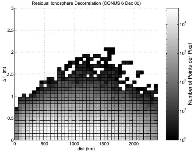
**Figure 1.** A two dimensional histogram representing the distribution of differential vertical delays, after a planar fit has been removed, versus IPP separation. This data is for a quiet day. The bar at the right indicates the number of counts per square.
