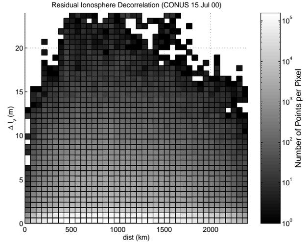
**Figure 2.** A two dimensional histogram representing the distribution of differential vertical delays, after a planar fit has been removed, versus IPP separation. This data represents a disturbed day.
