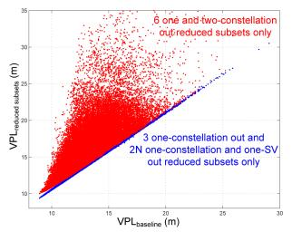
**Figure 2.** Relative performance of 6 one- and twoconstellation out subsets & 3 one-constellation out and 2N one-constellation and one-satellite out subsets vs. evaluating all first order (and second order as needed) subsets.
