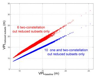
**Figure 3.** Relative performance of 6 two-constellation out subsets & 10 one- and two-constellation out subsets vs. evaluating all first order (and second order as needed) subsets.
