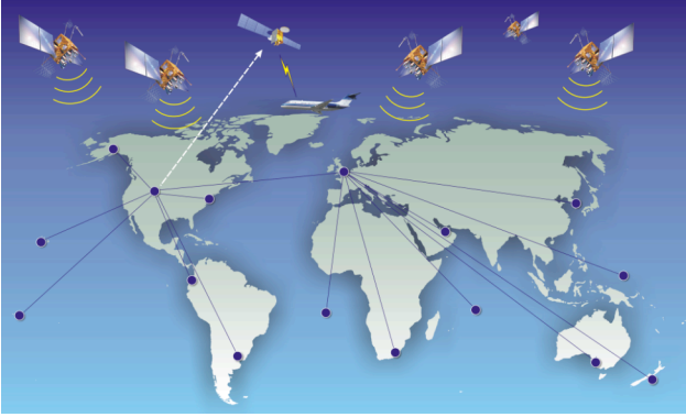
Figure 1. GIC Architectures. Here integrity is determined external to the aircraft and supplied within the TTA. Integrity may be determined either on the ground or on the satellites or through a combination of both. The integrity information may be broadcast through either geostationary satellite as in WAAS or via the GPS satellites themselves.
