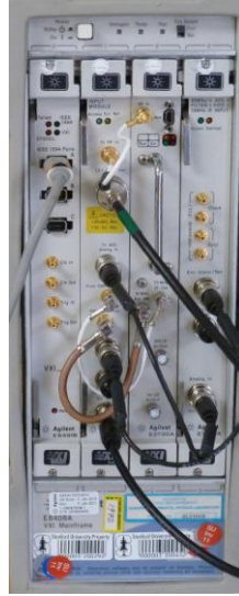
Figure 3-2: Agilent 89600 Vector Spectrum Analyzer (VSA), a high-rate, high-resolution, large bandwidth data logger
