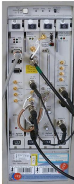
Figure B-2: Specialized data-collection equipment. Used to collect high-rate, high-precision raw baseband data
