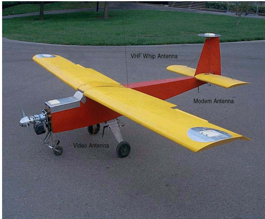
Figure 6.4. DragonFly Radio Frequency Equipment Locations
