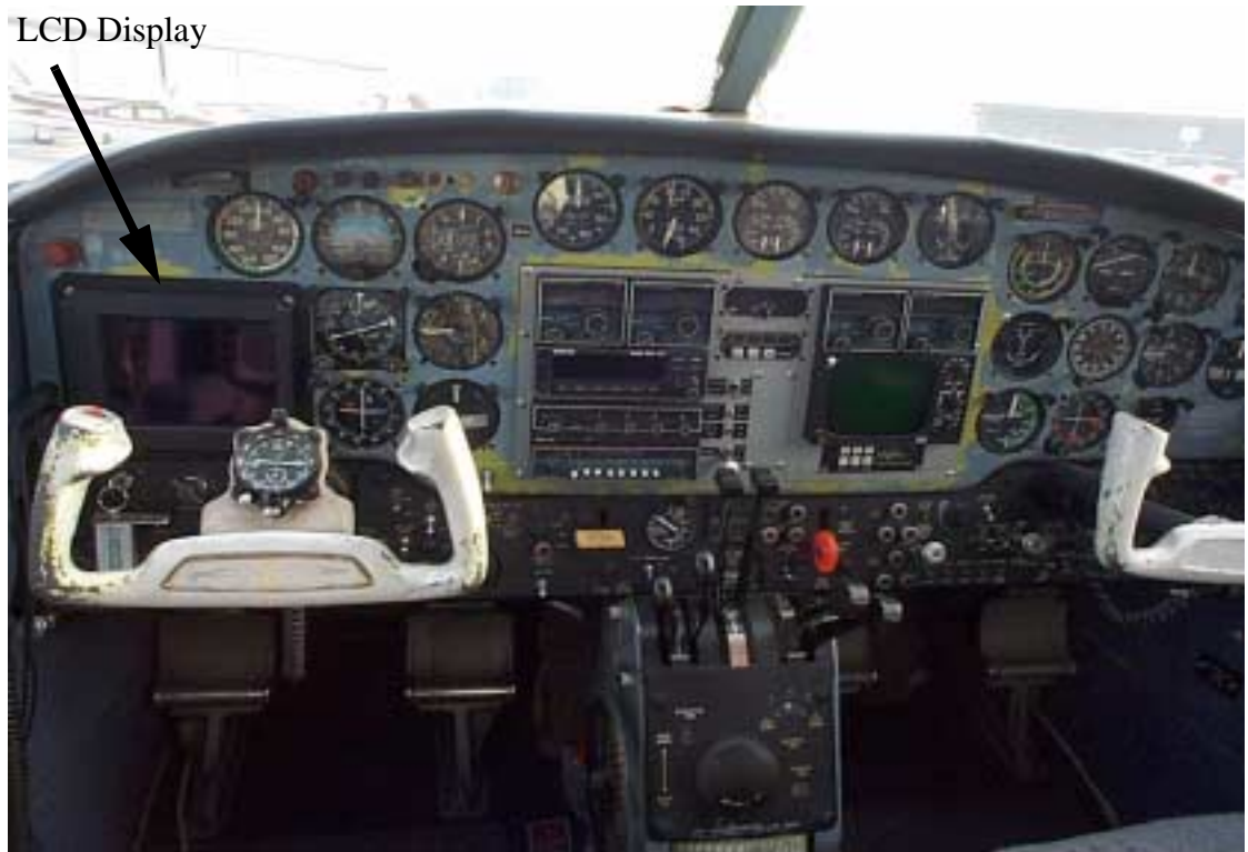
Figure 6-10. Cockpit of the Queen Air. Note the 6 inch LCD display to the pilot's left.
