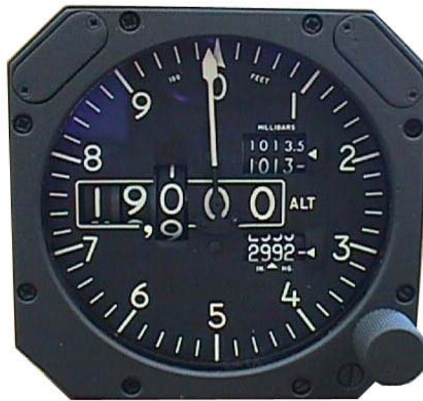
Figure 6.1: A barometric altimeter.
