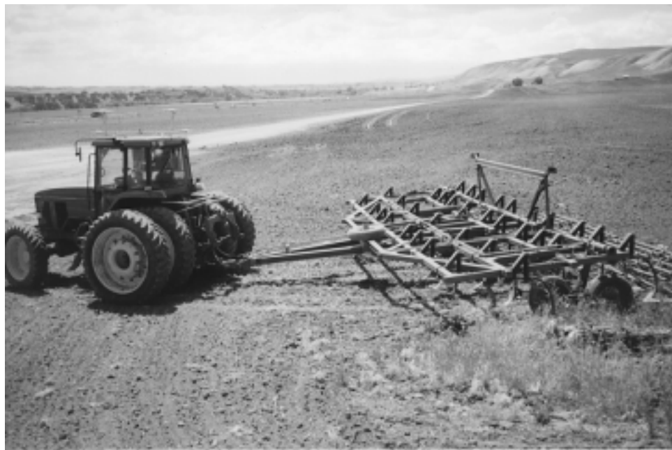
Figure 2.2: Chisel plow used for testing on the Model 7800. This particular towed implement was considered too large for the 7800.
