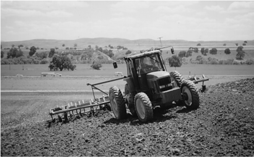
Figure 12.4: The tractor climbing over a sloped ridge. The tractor is actually approaching the photographer with a significant crab angle and steering bias.
