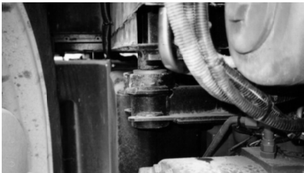
Figure 5.1: Photo of rubber mounts between tractor cab and frame. The camera is at the rear of the tractor looking forward. The inside of the left rear wheel can be seen on the left.
