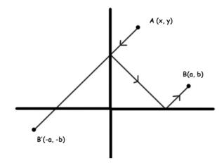
If you consider the mirror image of that light ray's path for both mirrors you get a second path of length equal to the actual path, which travels from (x,y) to (-a,-b) (as seen in the second picture). So the total length the light ray travels is the distance from (x,y) to (-a,-b). This would be  $\sqrt{(x+a)^2+(y+b)^2}$ .
