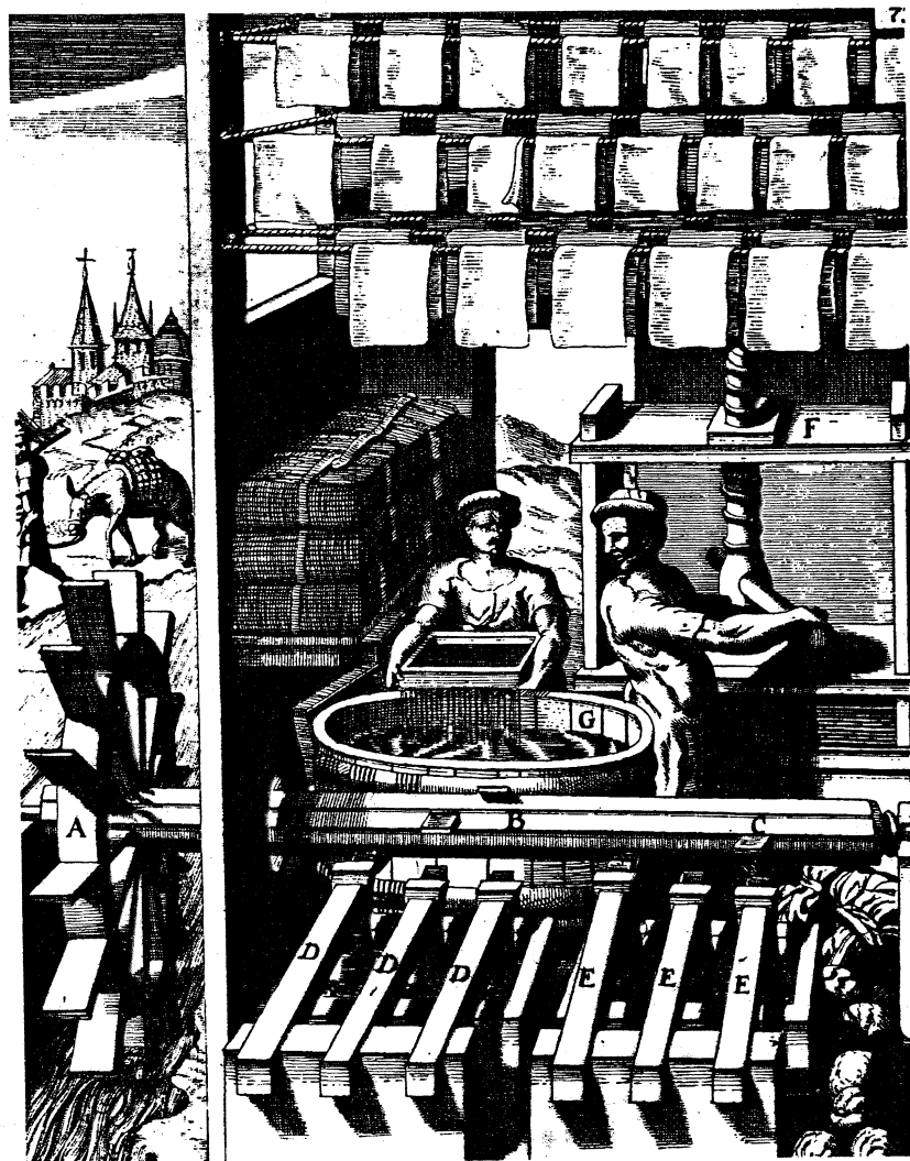
PAPER MILL relied on an undershot wheel with cams (c) to lift and drop hammers (d, e) that reduced rags to pulp. Thereafter the process was manual: the pulp was transferred to a vat (g), dipped out with a sieve and formed into a sheet in a press (f). The sheets were hung on racks to dry. The plate is from Georg Andreas Böckler's Theatrum machinarum novum of 1662.
