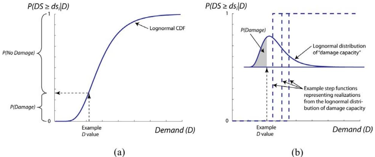
Figure 1: Two equivalent representations of an element fragility. (a) A lognormal CDF specifying the probability of collapse. (b) A step function specifying the probability of collapse, with the location of the step described by a lognormal distribution.
