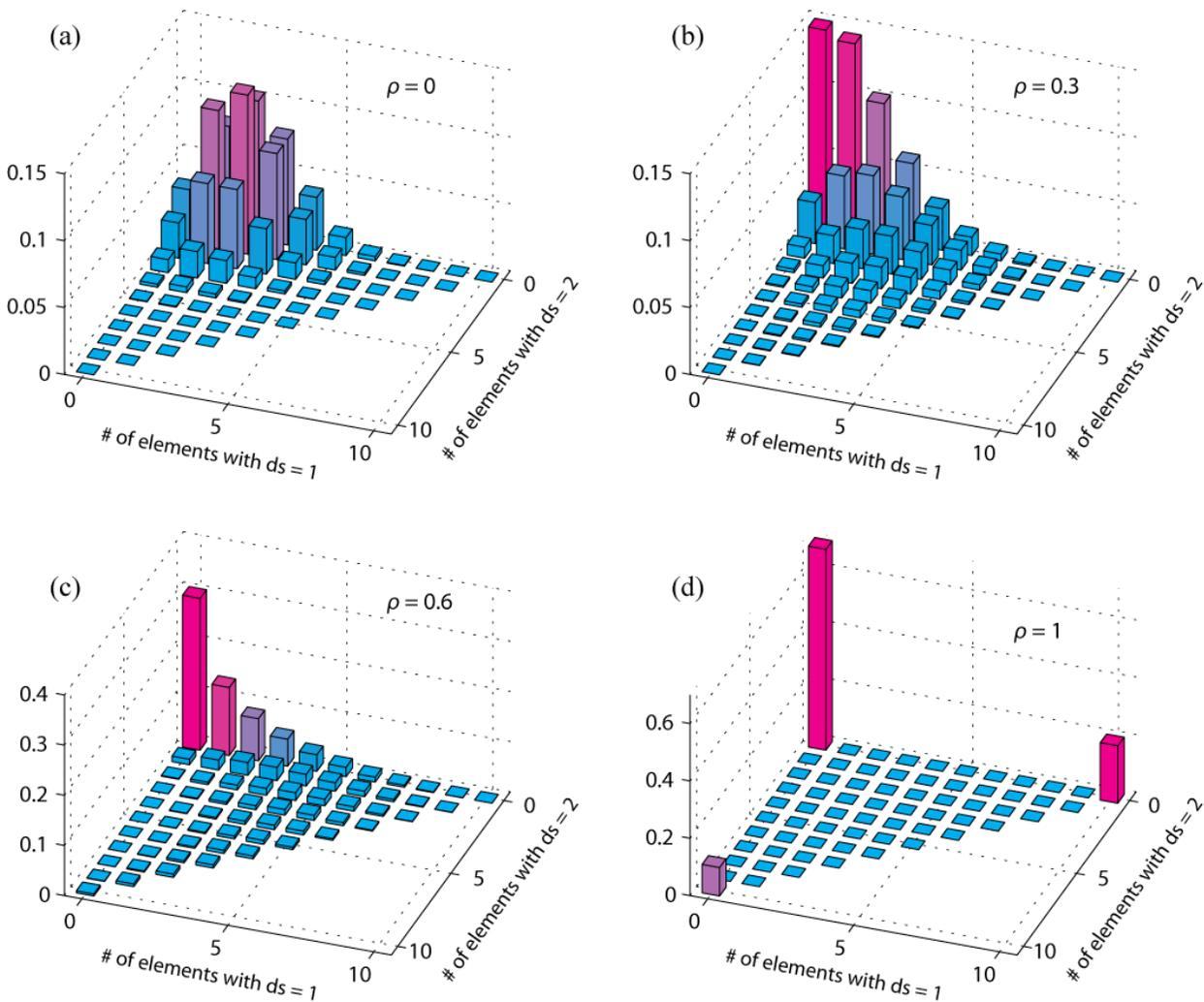
Figure 4: Probability of observing  $n$  damaged components out of 10, when there are two potential damage states and  $P(DS \geq 1) = 0.3$  and  $P(DS \geq 2) = 0.1$ , for four correlation coefficient values. (a)  $\rho=0$  (uncorrelated fragilities). (b)  $\rho=0.3$ . (c)  $\rho=0.6$ . (d)  $\rho=1$  (perfectly correlated fragilities).
