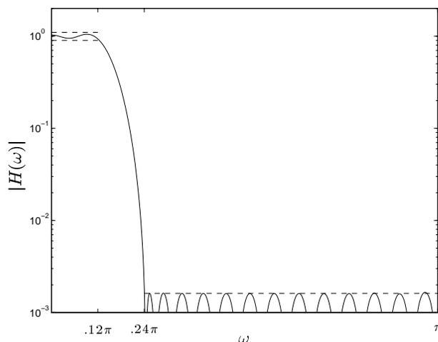
FIGURE 2. Maximum stopband attenuation design. The filter order is  $n = 30$ , maximum passband ripple is  $\alpha = 1.1$  (about 1dB), passband frequency is  $\omega_p = 0.12\pi$ , and stopband frequency is  $\omega_s = 0.24\pi$ . The stopband attenuation achieved is  $-56\text{dB}$ .
