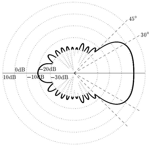
FIGURE 10. Example of antenna array weight design for 12-element array with spacing  $d = 0.45\lambda$ . The constraints require  $\pm 2$ dB coverage over a beam of  $\pm 30^\circ$  and the objective is to minimize the maximum pattern response outside a  $\pm 45^\circ$  sector. The sidelobe level achieved is about  $-19$ dB.
