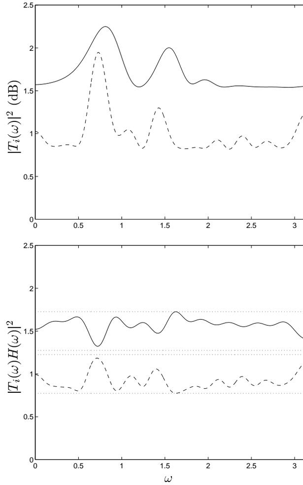
FIGURE 7. Example of multi-system magnitude equalization. The two frequency response squared magnitudes  $|T_1|^2$  (solid) and  $|T_2|^2$  (dashed) are shown in the upper plot. The equalized frequency response magnitudes  $|T_1H|^2$  (solid) and  $|T_2H|^2$  (dashed) are shown in the lower plot, along with the ranges  $\gamma_{\text{opt}} \pm \alpha_{\text{opt}}$  (dotted).
