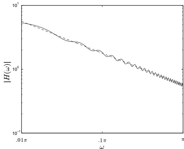
FIGURE 3. Magnitude frequency response of a 50th order  $1/f$  spectrum shaping filter for frequency range  $[0.01\pi, \pi]$ . Dashed line shows ideal  $1/\sqrt{f}$  magnitude, which falls at 10dB/octave. The maximum approximation error is  $\pm 0.5$ dB.
