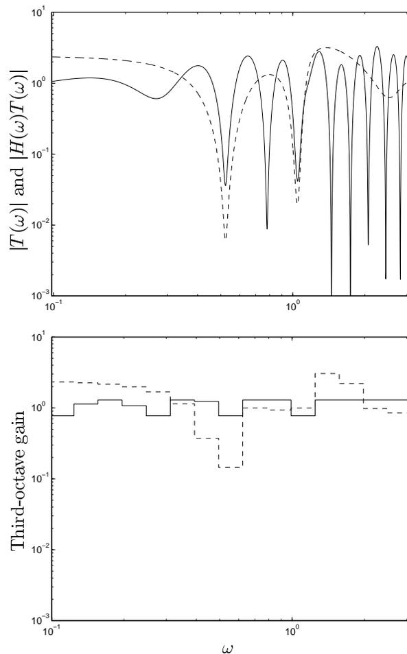
FIGURE 8. Example of third-octave equalization, with constraint that equalizer frequency response magnitude not exceed 10. Upper plot shows  $|T|$  (dashed) and the equalized frequency response  $|TH|$  (solid). Lower plots shows third-octave gains for  $T$  (dashed) and  $TH$  (solid). The third-octave gains have been equalized within  $\pm 1.1$ dB. Since  $|T|$  is small at several frequencies, ordinary log-Chebyshev equalization to  $\pm 1.1$ dB would require very large values of  $|H|$ .
