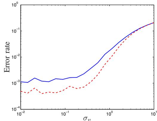
**Fig. 3:** Average error rate in  $z$  for the RMAP estimate with (dashed) and without (solid) local optimization.
