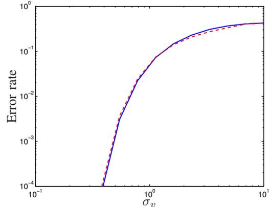
**Fig. 2:** Average error rate as a function of  $\sigma$  for the RMAP estimate (solid) and the true MAP estimate (dashed).
