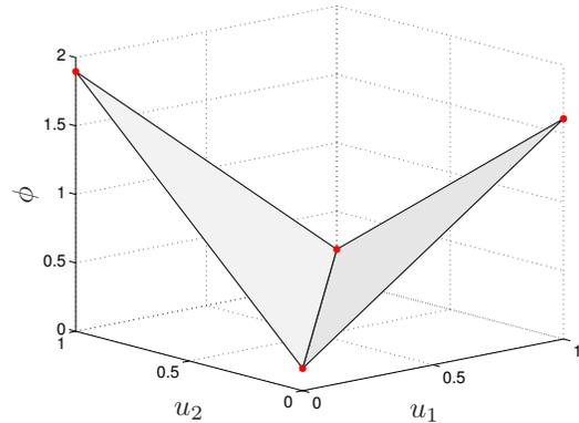
**Fig. 1:** Graph of convex envelope  $\bar{\phi}$  (shaded planes) and  $\phi$  (the four points shown as balls) for  $p^{\text{up}} = 0.15$  and  $p^{\text{down}} = 0.2$ . This corresponds to the first case described below, since  $[q_{00}, q_{11}]$  lies below  $[q_{01}, q_{10}]$ .
