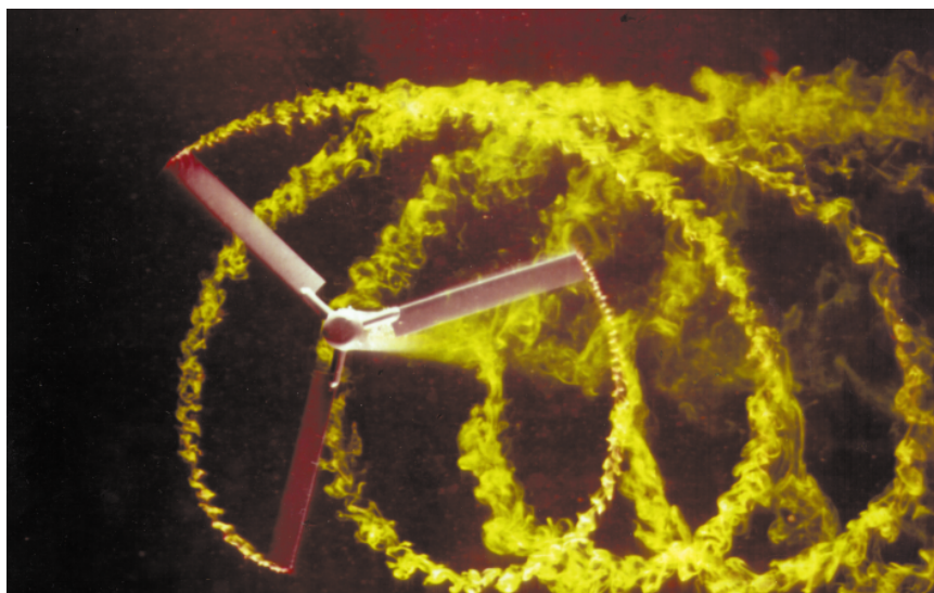
Figure 2 Tip vortices emanating from the blades of a helicopter rotor.
