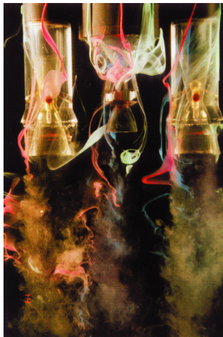
Figure 3 Flow in the base region of the Ariane 5 space launcher.
