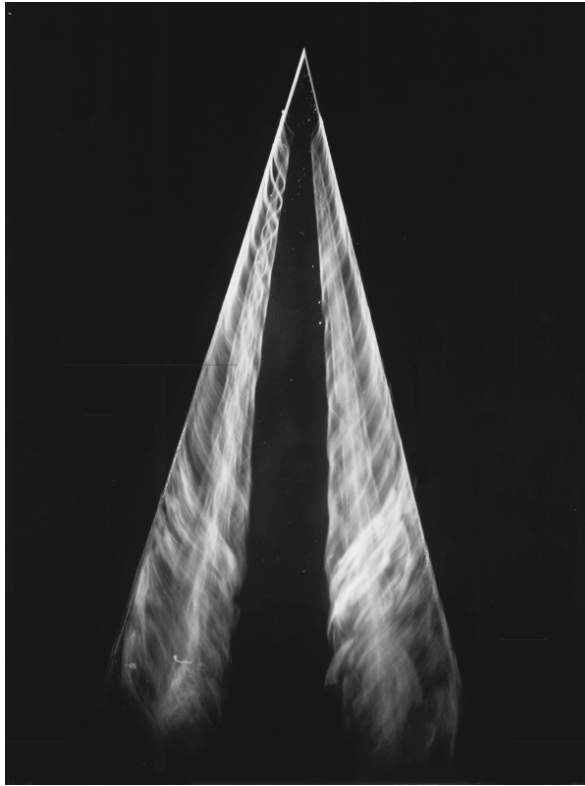
Figure 9 Vortices over a 75^\circ -sweep angle delta wing.
