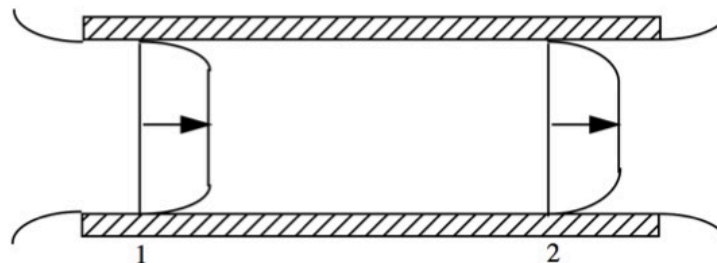
Figure 5.11: Steady flow in an empty wind tunnel
