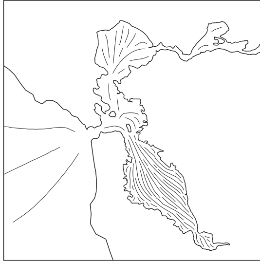
Figure 13. Flow-aligned contours, traced from the principal velocities, ready for input to the regridding process. The separation between adjacent contours scales with the grid resolution, leading to sparser contours in the north and west.
