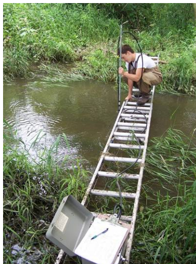
Figure 51: Typical Flowrate Measurement (J. Anderson at Ripp Gage)
