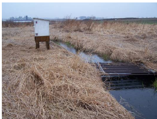
Figure 40: Dorn Gage Site, Showing Sampler Housing (March 2006)
