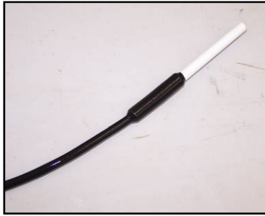
Figure 52: Campbell Scientific T-107 Temperature Sensor
