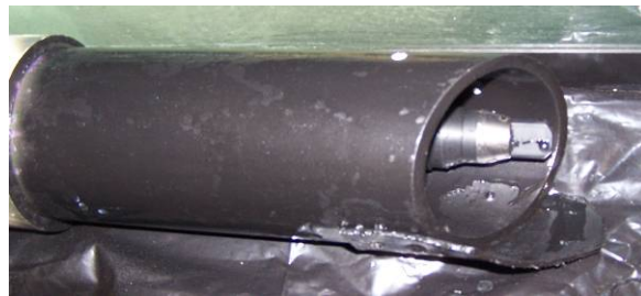
Figure 46: OBS-3 Probe with Protective Stilling Well Pipe
