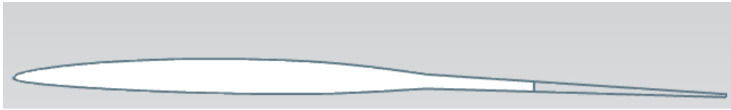
Figure 7.8.58: Airfoild Section of the wind tunnel model
