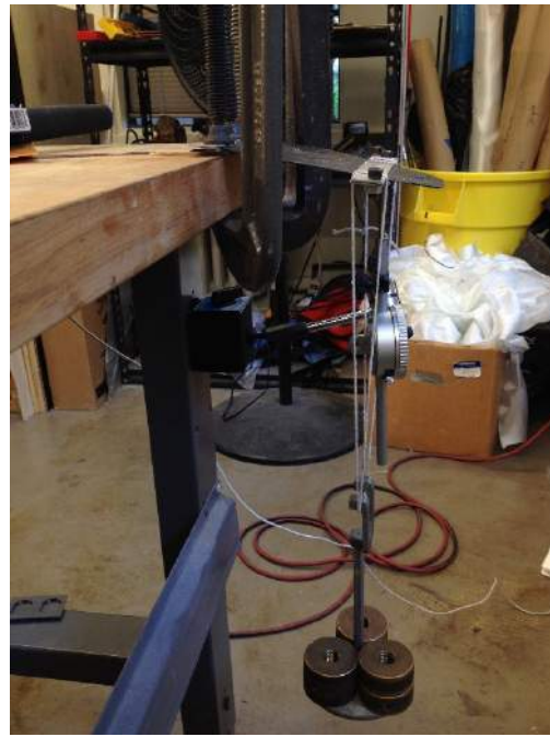
(2) Carbon-foam Canard Deflection w/ Heavier Weight
