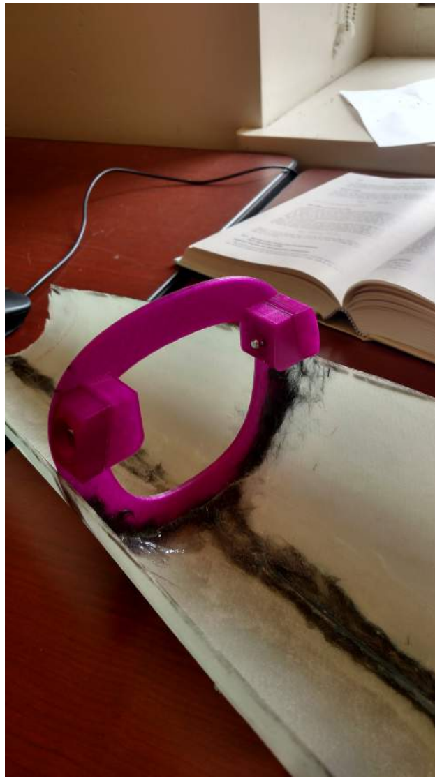
Figure 5.3.4: The image above shows a 3D printed bulkhead that was mocked up in a short fuselage section made with 2014's molds.
