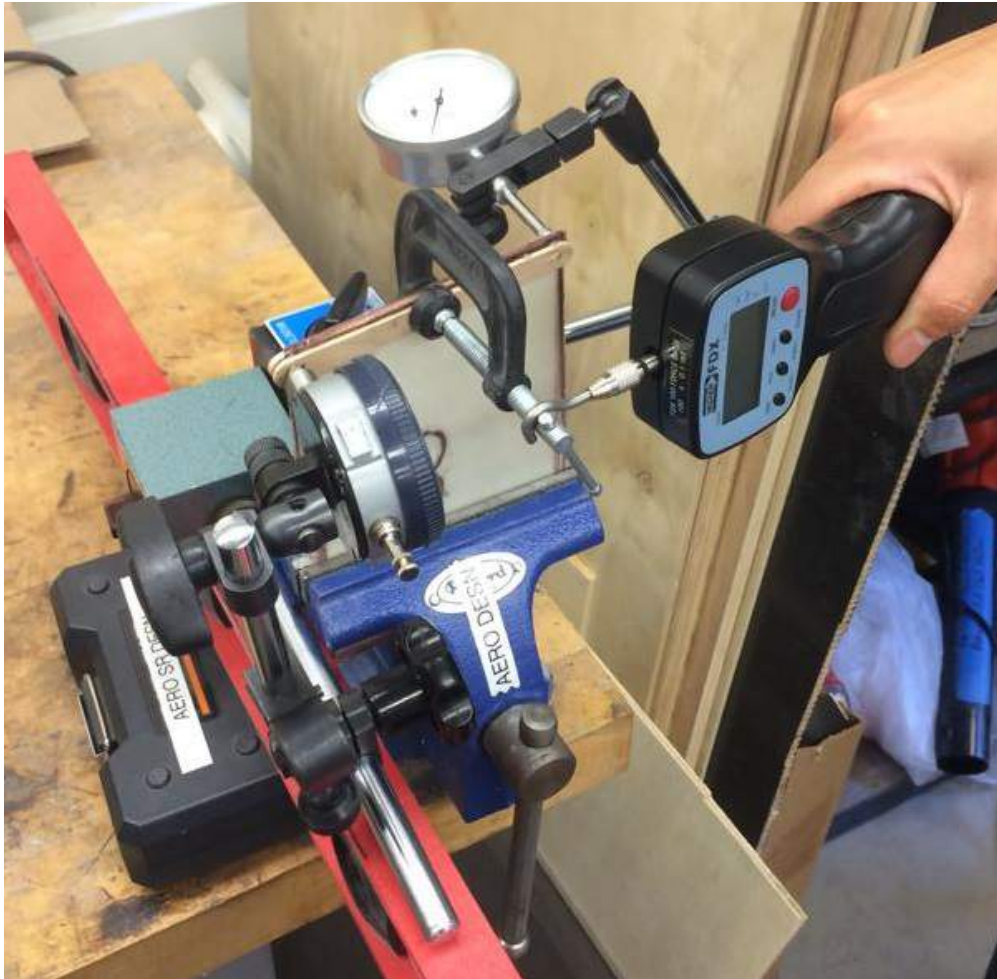
Figure 7.1.7: The actual torsion test setup used.
