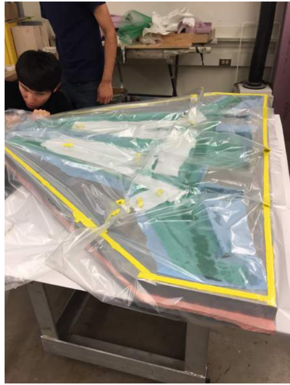
(2) Process of securing the vacuum
