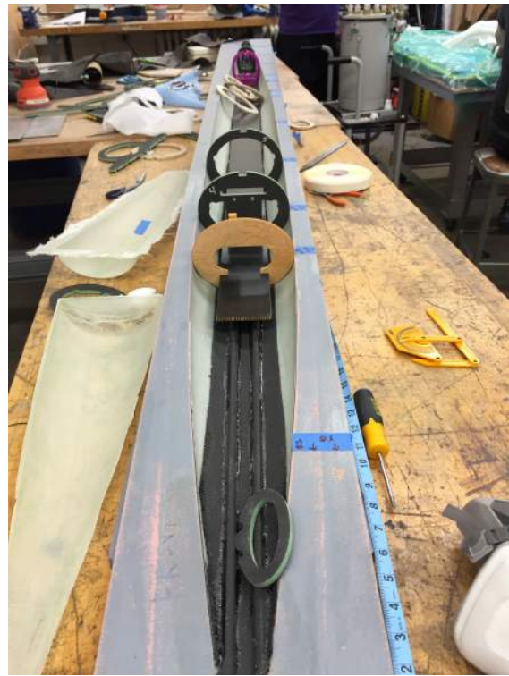
(2) Keel Beams of the fuselage reinforcement
