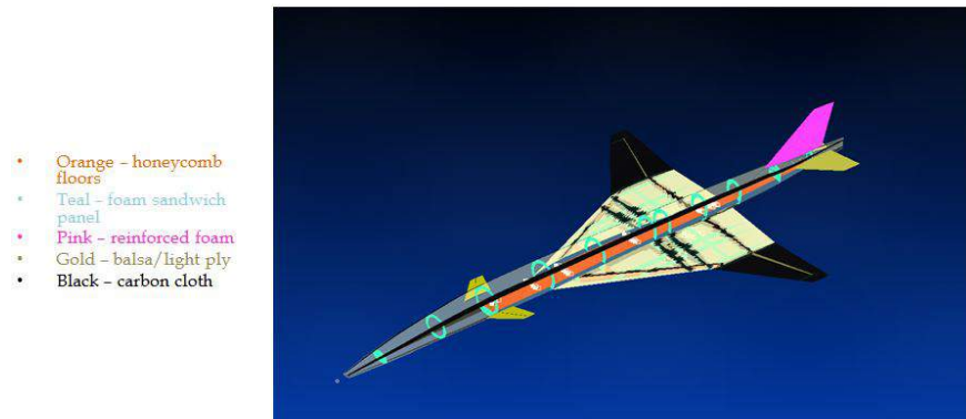
Figure 7.1.30: A breakdown of which materials were used in FEMAP and the final aircraft.
