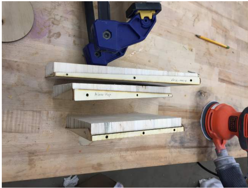
Figure 7.9.5: Balsa wood with templates used to shape them.
