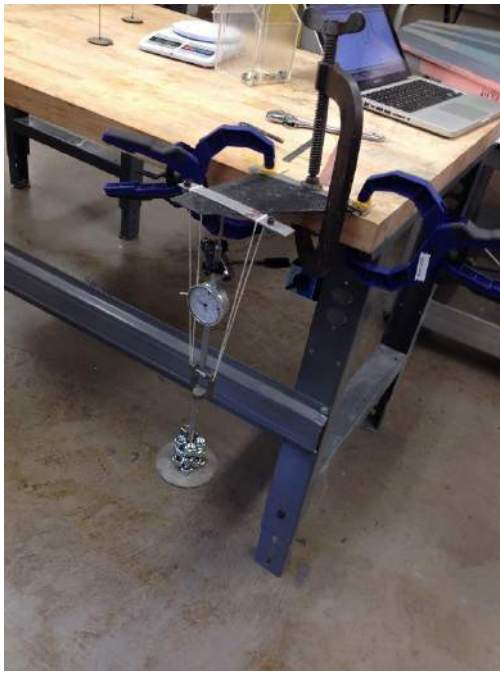
(1) Carbon-foam Canard Deflection w/ Light Weights
