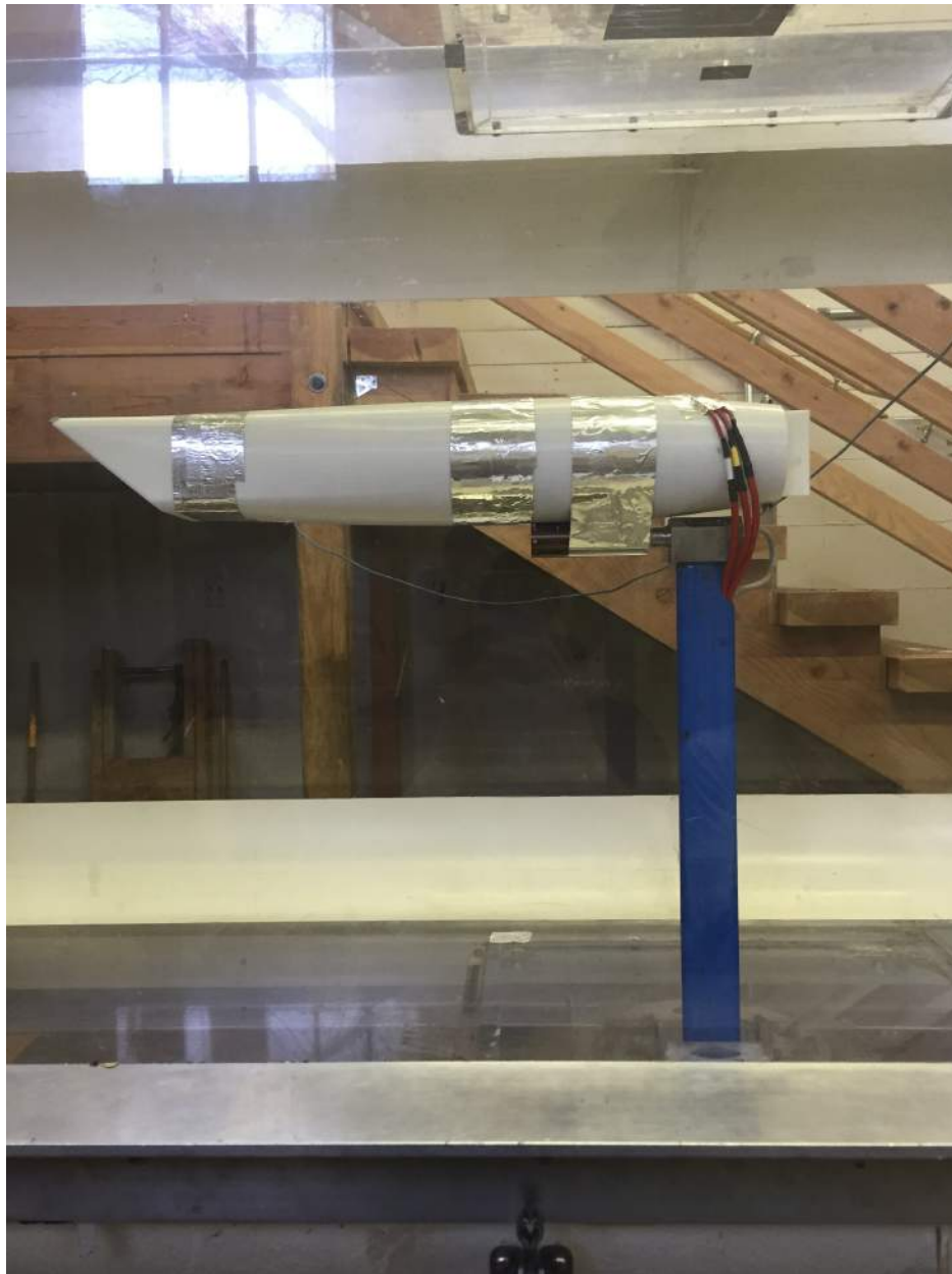
Figure 6.2.1: Set up of the nacelle in the 3 \times 3 wind tunnel
