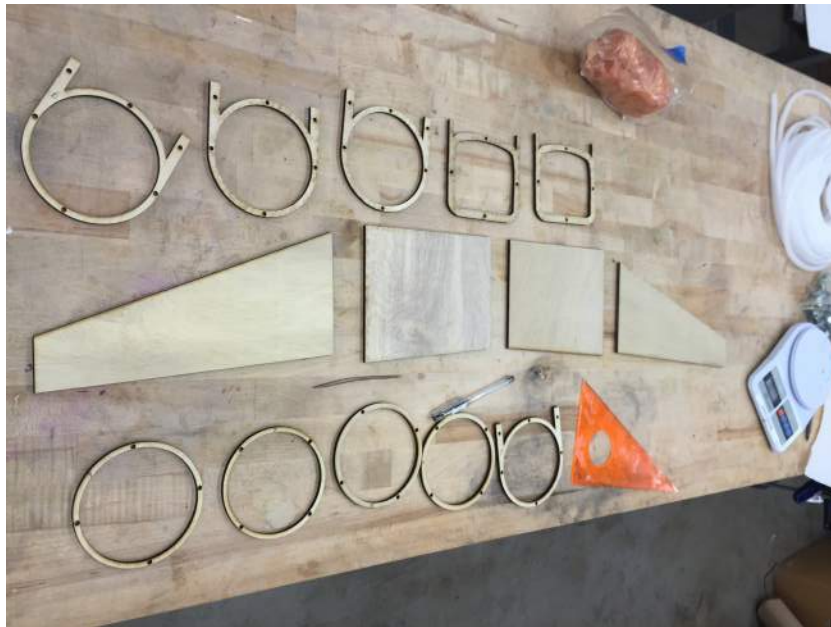
Figure 7.9.8: Laser cut nacelle bulkheads
