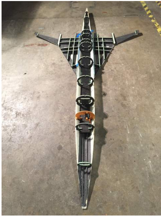
Figure 7.9.11: The internal structure of the R-UAV
