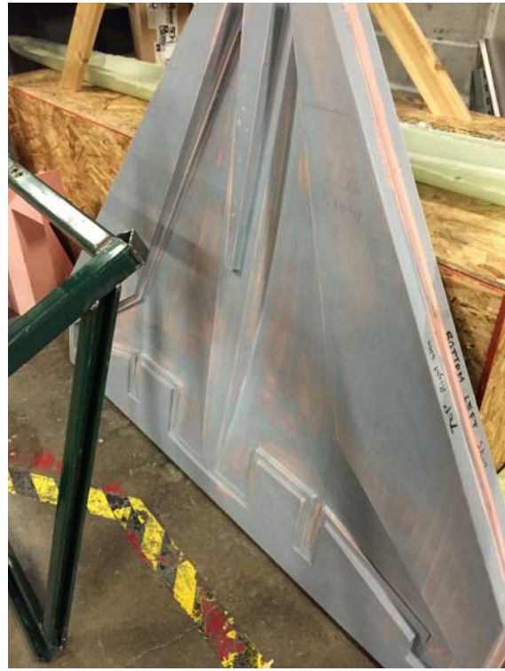
(2) R-UAV wing molds
