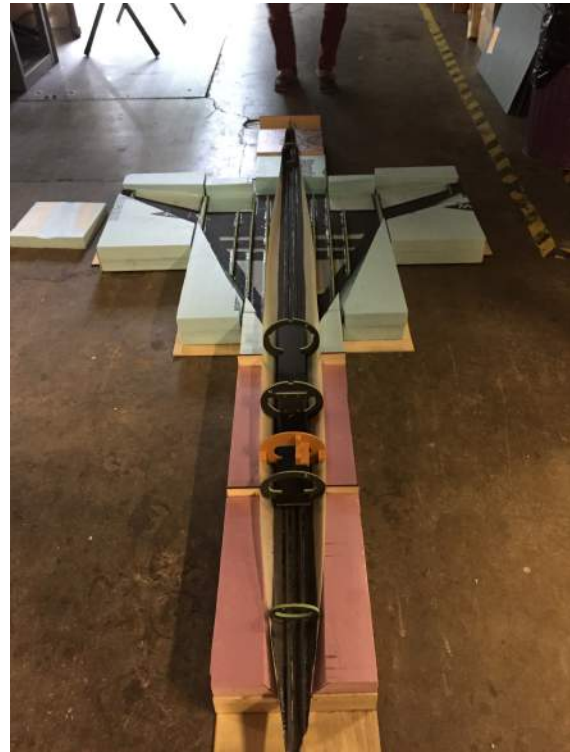
(2) Keel Beams of the fuselage reinforcement
