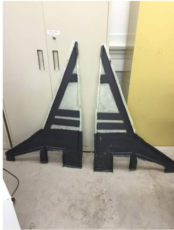
(2) Final carbon fiber arrangement along the wings
