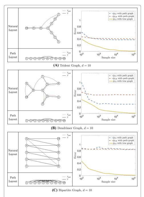
**Fig. 8** The black solid line stands for edges on T and the dashed brown line stands for edges on  $T_{\rm path}$ . The graph is plotted in a layout that is respectively natural for T and for  $T_{\rm path}$ . Error plots for each case of T are also included. One can see that convergence to the true model only occurs with true tree specification
