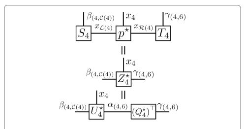
**Fig. 4** Tensor diagram of the sketching step in (12) and the SVD step in (13). The illustration is over the rooted tree in Fig. 2
