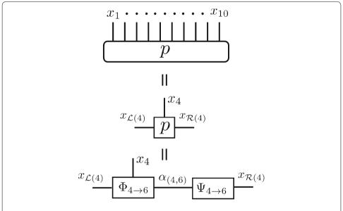
Fig. 3 Tensor diagram representation of the TTNS ansatz assumption in Condition 1. The illustration is over the rooted tree in Fig. 2 with (w, k) = (4, 6). The symbol  $x_{\mathcal{L}(4)} = (x_1, x_2, x_3, x_5)$  and  $x_{\mathcal{R}(4)} = (x_6, x_7, \dots, x_{10})$  is a short-hand for joint variables as defined in Definition 4
