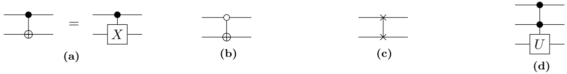
Fig. 2. (a) CNOT gate. (b) |0\rangle -controlled-NOT gate. (c) SWAP gate. (d) An example of a multi-qubit control gate |11\rangle\langle 11| \otimes U + (I_4 - |11\rangle\langle 11|) \otimes I . The two filled nodes indicate that U is applied to the third qubit if and only if both the first two qubits are at state |1\rangle .
