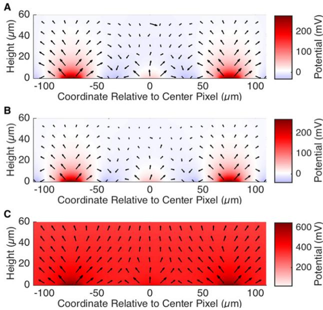
**Figure 11.** Potential (color map) and current (arrows) above the central three pixels in the middle row of the array for isolated (A), connected (B), and monopolar (C) return configurations. Central pixel is ‘dark’ (current  $I_{\min} = 0.2 \mu\text{A}$ ) and adjacent ones are ‘bright’ (current  $I_{\max} = 1 \mu\text{A}$ ) in the grid pattern. Arrays with local returns confine the current and potential above the device much better than the monopolar configuration with the same input.
