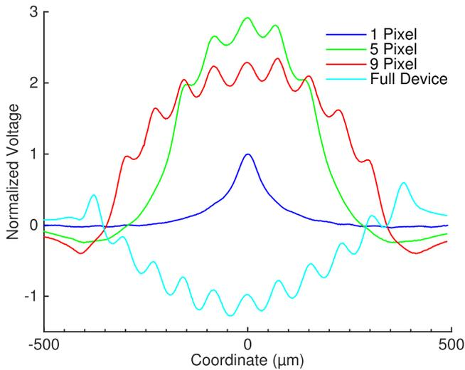
**Figure 8.** Experimentally measured potential in the medium above the photovoltaic array for various beam sizes, normalized to potential above the single illuminated pixel. Widening the spot from 1 to 5 pixels increases the potential, but further beam expansion decreases it.
