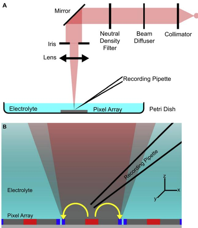
**Figure 2.** Diagram of the setup for measuring electric potential above the array. (A) Laser beam projected via the microscope. (B) Laser beam illuminating a single photovoltaic pixel in the array. Recording pipette translated laterally with  $2\ \mu\text{m}$  steps to map electric potential in the medium.
