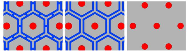
**Figure 3.** Three configurations of the return electrodes: left—connected local returns; middle—disconnected local returns; right—common remote return electrode on the back surface of the array.
