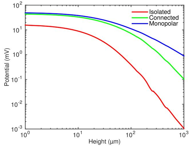
**Figure 12.** Potential as a function of height above the single activated pixel. One millimeter above the array, a pixel with isolated returns generates a potential three orders of magnitude lower, and with connected returns—1 order of magnitude lower than that of a monopolar pixel (1  $\mu\text{V}$  100  $\mu\text{V}$ , and 1 mV, respectively).
