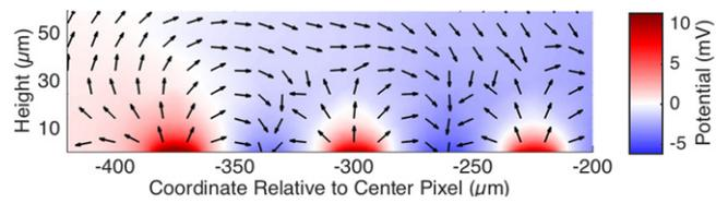
**Figure 10.** Potential (color map) and current (arrows) above the three peripheral pixels in the central row of the array. Due to reduced capacitance of the local return electrode at the edge of the array, peripheral pixels cannot locally return their injected current, and it flows towards the more central areas. This effect increases the negative potential of the returns in the center.
