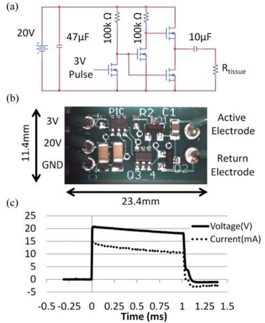
Fig. 6. (a) Miniature stimulator circuit schematic. (b) Stimulator assembled on a PCB of  $11 \times 23$  mm in size. (c) Voltage and current output waveforms of the device with tissue load (average,  $n = 4$ ).
