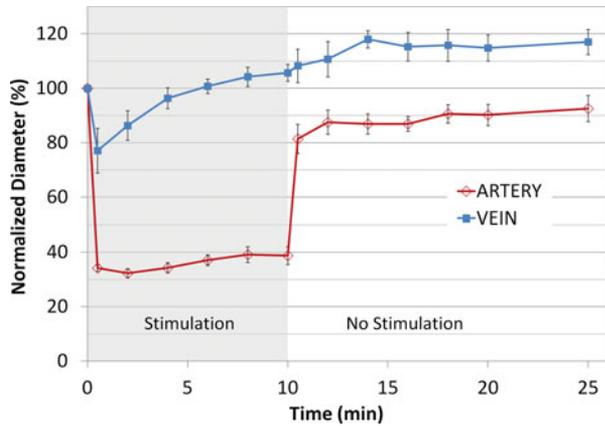
Fig. 7. Vessel constriction using miniature stimulator. The artery constricted to  $34 \pm 1\%$ , similar to the response obtained with the bench-top pulse generator (see Fig. 1 and Fig. 2). The vein constricted only transiently. Error bars show SEM.
