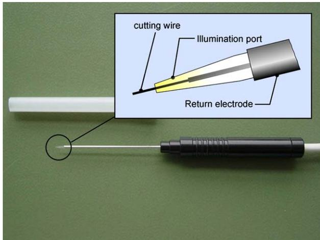
**Figure 1.** Diagram of PEAK-fc probe. The cutting part of the PEAK-fc probe is a protruding Tungsten wire with a diameter of 50  $\mu\text{m}$ . The wire used in this study extends from the glass insulator 0.6 mm in length.
