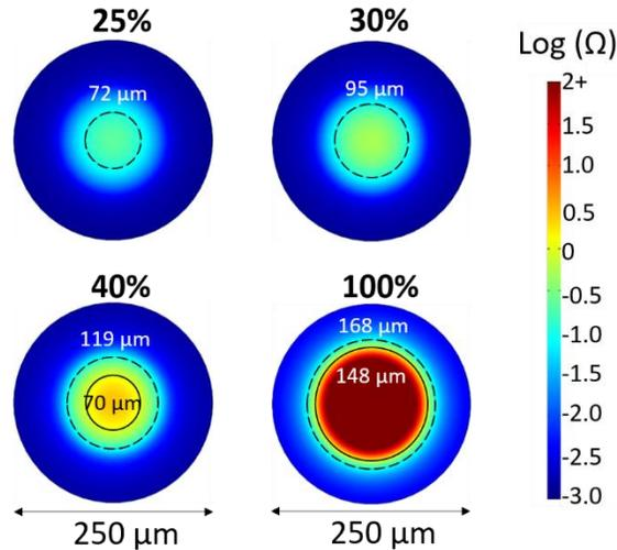
Figure 6. Arrhenius integral calculations for HSP expression and damage threshold. Dashed line indicates  $\Omega = 0.1$  where HSP expression is expected to begin. Solid line indicates  $\Omega = 1$  where cellular damage is expected.
