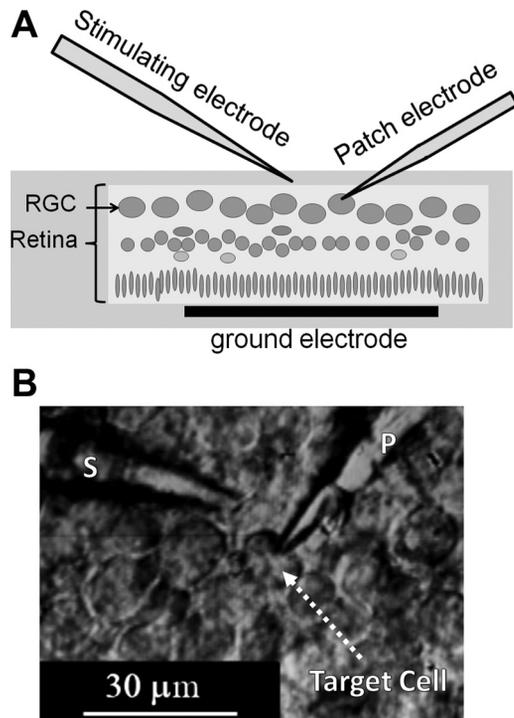
Fig. 1. In vitro patch-clamp recording from retinal ganglion cells (RGCs) in the isolated retina during extracellular stimulation. *A*: schematic diagram of stimulation and recording. *B*: differential interference contrast microscope image of the RGC layer. A 1- to 2- $\mu\text{m}$  patch pipette (P) is attached to the target cell; the 4- $\mu\text{m}$  stimulation pipette (S) is held near the cell.
