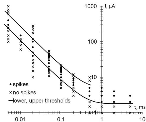
Fig. 4. Strength-duration dependence of the upper and lower thresholds of stimulation for rectangular cathodic pulses. The stimulation range (spikes, ●) lies between the lower and upper stimulation thresholds. No APs are elicited outside this range (no spikes, ×). The lower and upper thresholds are defined as having a 50% elicitation probability. The number of independent data points shown is 86;  $\tau$ , stimulus duration.
