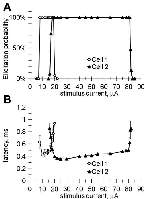
Fig. 3. Spiking elicited by 0.1-ms cathodic pulses as a function of the stimulus current shown for 2 different RGCs located at different distances from the stimulating electrode. *A*: probability of eliciting the APs. *B*: latency of elicited AP. Error bars correspond to the standard deviation of successive recordings. The number of independent data points shown for cell 1 is 14 and for cell 2 is 21.
