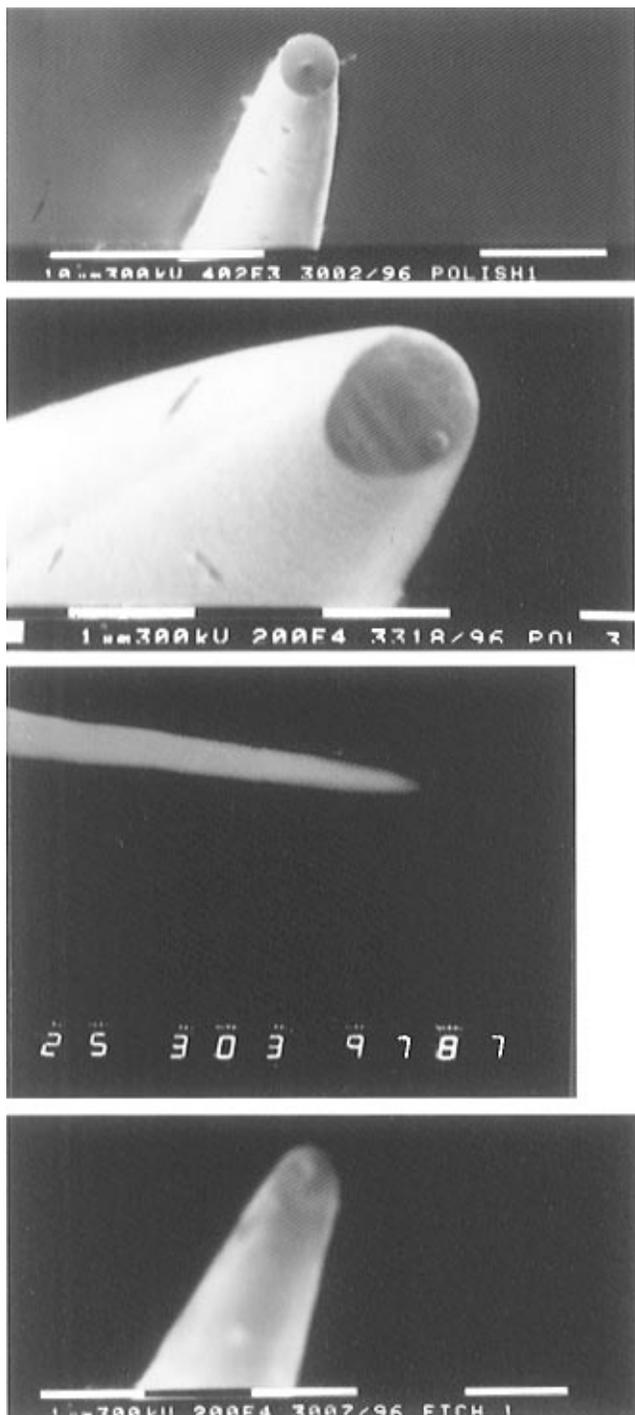
Figure 5. Scanning electron micrographs of submicrometer-sized tips. Top to bottom: (A) 150-nm-radius polished Pt UME; (B) 50-nm-radius conductive disk somewhat displaced toward the edge of the 1- $\mu\text{m}$ -radius glass ring; (C) Pt wire obtained by stripping  $\sim 1 \mu\text{m}$  of glass from the unpolished Pt UME; and (D) etched UME.
