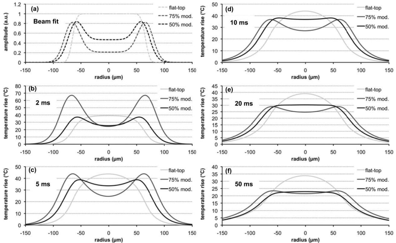
**Fig. 7** (a) Average functional fit [Eq. (3)] to measured beam irradiance for flat-top, 50% modulated annular beam, and 75% modulated annular beam, in arbitrary units (a.u.). (b–f) Computed maximum temperature rise for 2–50 ms durations. Mean threshold powers for mild coagulation with each beam shape were used in calculation of temperature.
