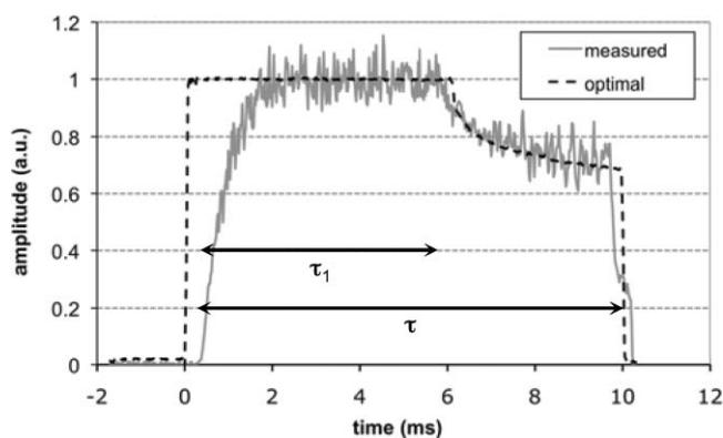
**Fig. 2** Computed optimal (dashed line) and measured experimental modulated power pulse shapes for 10-ms duration, in arbitrary units (a.u.). The measured pulse shape follows the optimal driving waveform closely, excluding the rise and fall periods.
