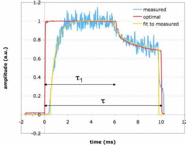
Fig. 1. Computed optimal (red), measured experimental (blue), and fit to experimental (yellow) pulse shapes for 10 ms duration.
