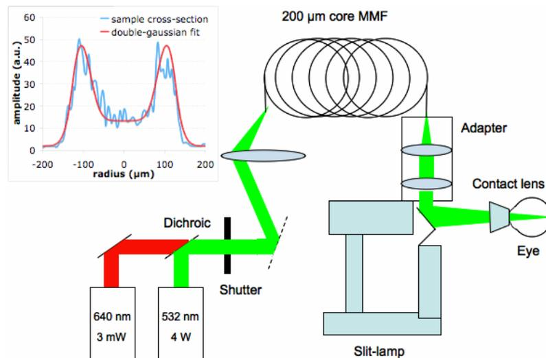
Fig. 2. Schematic for ring-beam photocoagulation setup. Ring-mode excitation is achieved through coupling into the multimode fiber (MMF) at an angle. A low-power 640 nm laser is coupled into the same mode for use as an aiming beam. A conventional slit lamp and fiber coupler serve as the delivery system. Inset: Sample aerial beam cross-section (blue) from experiments, with average functional fit (red) from Eqn. 4 used in computational modeling.
