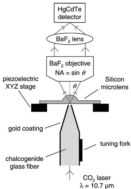
FIG. 1. Experimental setup used for refraction contrast imaging with a scanned Si microlens showing the stationary chalcogenide glass fiber source and BaF<sub>2</sub> objective with maximum collection angle  $\theta=46.7^\circ$  (NA=0.45).
