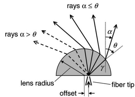
FIG. 3. Refraction of rays emitted at angles  $\gamma$  from a source that is offset from the geometrical center of the lens. Rays refracted at angles  $\alpha$  less than the maximum collection angle  $\theta$  are collected (solid), while lines with angles  $\alpha$  greater than  $\theta$  are not (dashed).
