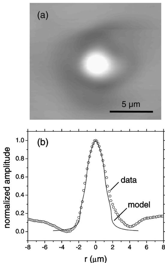
FIG. 2. (a) Refraction contrast image of the  $\lambda/10$  tapered fiber tip taken with a scanning 10- $\mu\text{m}$ -diameter Si microlens. (b) Normalized line scan through the image. The solid line plotted with the data is the result of a three-dimensional model of refraction in the lens with an offset in lens thickness equal to 10% of the diameter.
