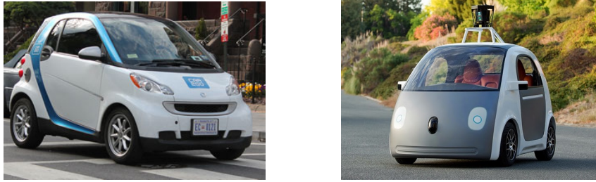
Fig. 19.1 Left figure: A Car2Go vehicle used in a traditional (i.e., non-robotic) MoD system. Right figure: Self-driving vehicle that Google will use in a 100-vehicle AMoD pilot project within the next two years. Image credit: Car2Go and Google.
