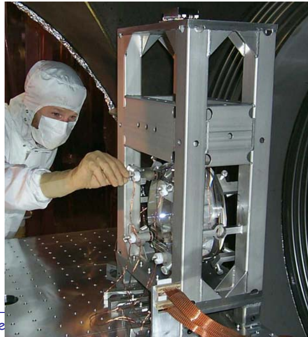
Fused Silica, 10 kg, 25 cm diameter and 10 cm thick Polished to \lambda/1000 (1 nm)
