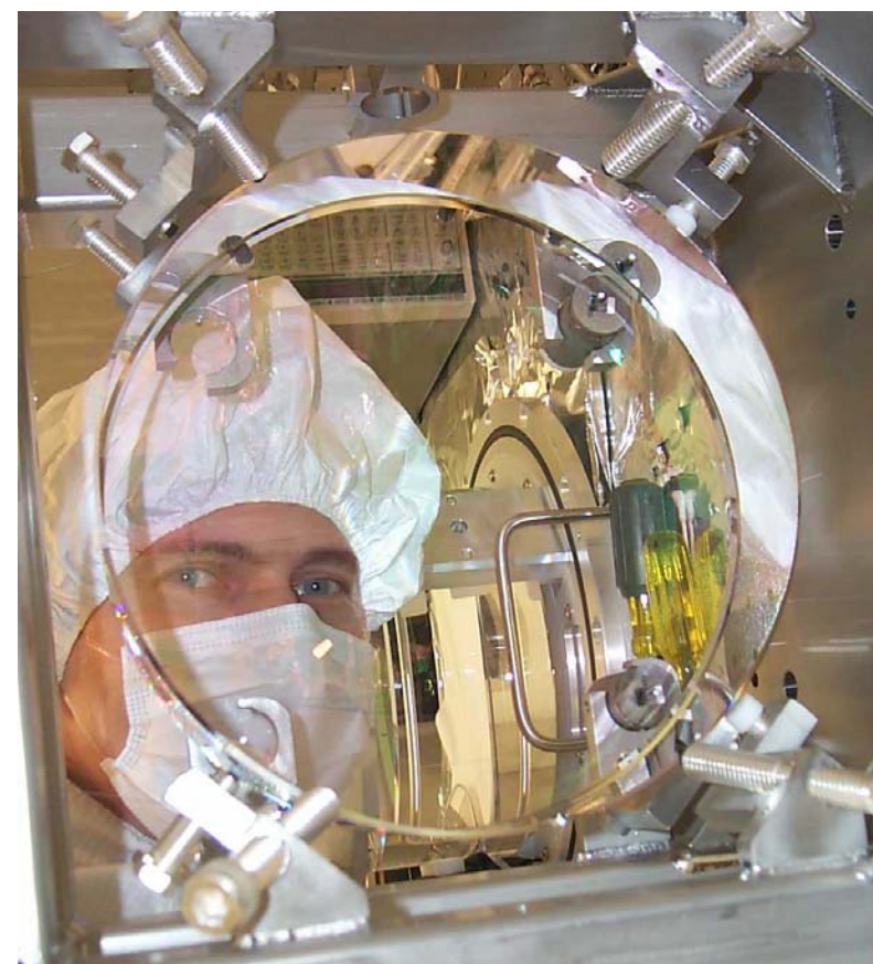
Fused Silica, 10 kg, 25 cm diameter and 10 cm thick Polished to \lambda/1000 (1 nm)
