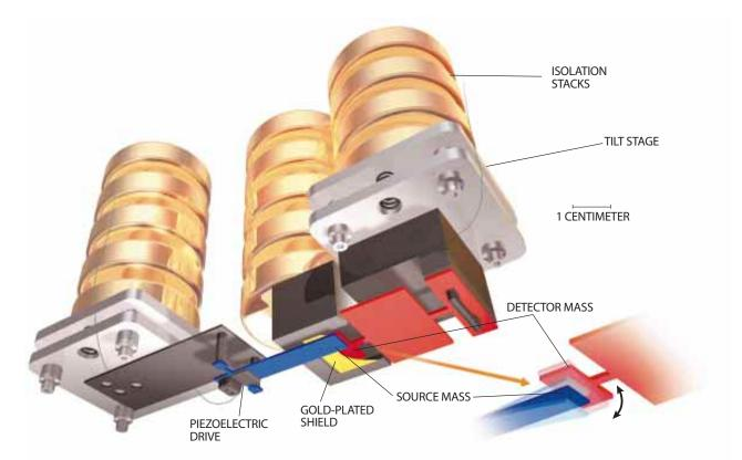
TORSION OSCILLATOR at the University of Colorado looks for changes in gravity from 0.05 to 1.0 millimeter. Piezoelectrics vibrate the tungsten source mass (*blue*) like a diving board. Any forces acting between the source mass and the tungsten detector (*red*) produce twisting oscillations of the detector (*inset*; *oscillations are exaggerated*), which are sensed by electronics. A gold-
