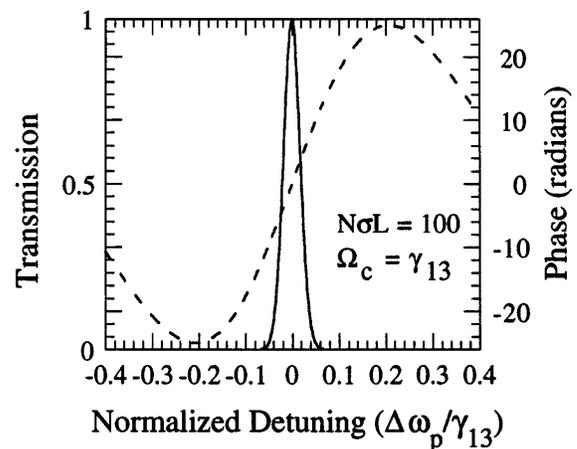
FIG. 1. Transmission and phase of the probe with perfect EIT.
