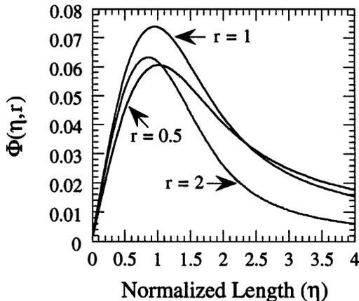
FIG. 3.  $\Phi(\eta, r)$  vs normalized length. The function  $\Phi(\eta, r)$  is evaluated for Gaussian pulses of equal length.
